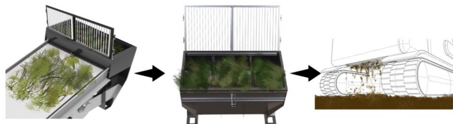
Figure 10. Spartina alterniflora recovery and sieve out impurities process.
