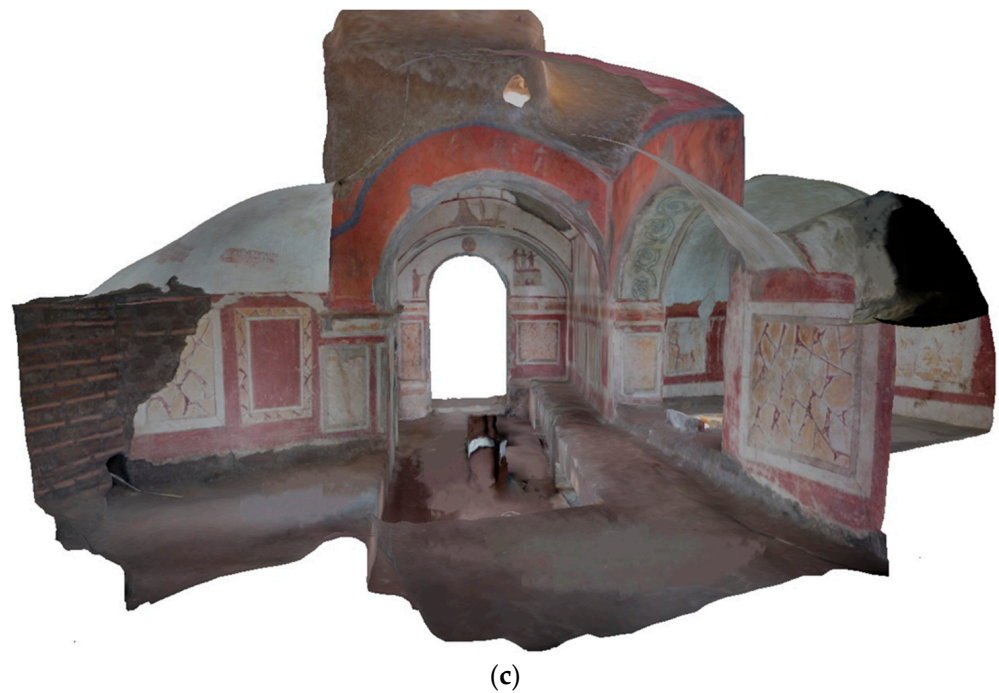
Figure 7. Three-dimensional model of the Greek chapel obtained with the RGB-ITR laser scanner: (a) view of the mesh where the room geometry is clearly visible and the investigated area is indicated; (b,c) sections of the model where all the room can be viewed and the accurate colours of the texture allow to better appreciate the paintings.
