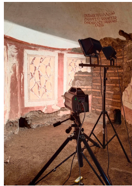
Figure 6. Thermographic apparatus working in the chapel.
