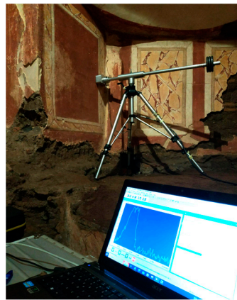
Figure 3. NMR system during the acquisition process.
