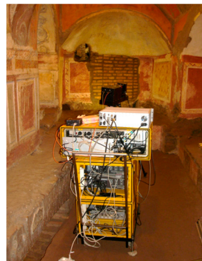
Figure 2. RGB-ITR scanner at work inside the Greek chapel.
