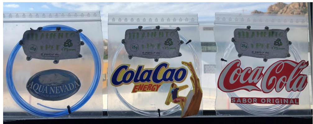
Figure 5. rPET filament produced from 1.5 L PET bottles.
