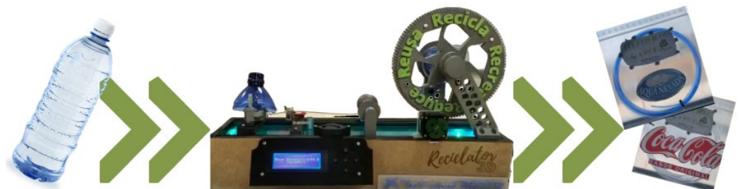
Figure 4. rPET filament production process via pultrusion.
