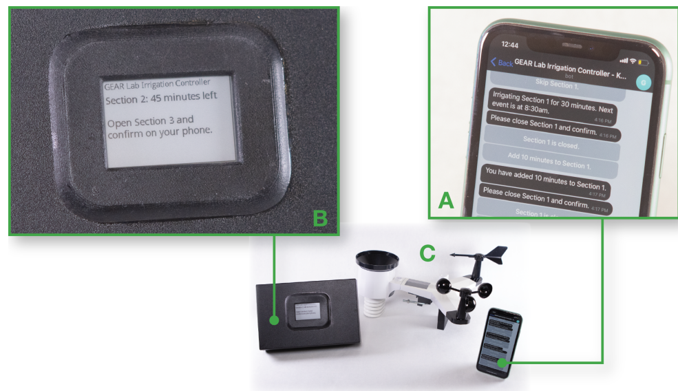
Figure 3. The three components of the physical prototype used to facilitate interviews. The phone (A) was equipped with a Telegram bot that stepped farmers through a set of key interactions. The control box (B) displayed the status of these interactions and directed farmers to interact on the phone. The low-cost weather station (C) showed farmers what data the tool might collect.
