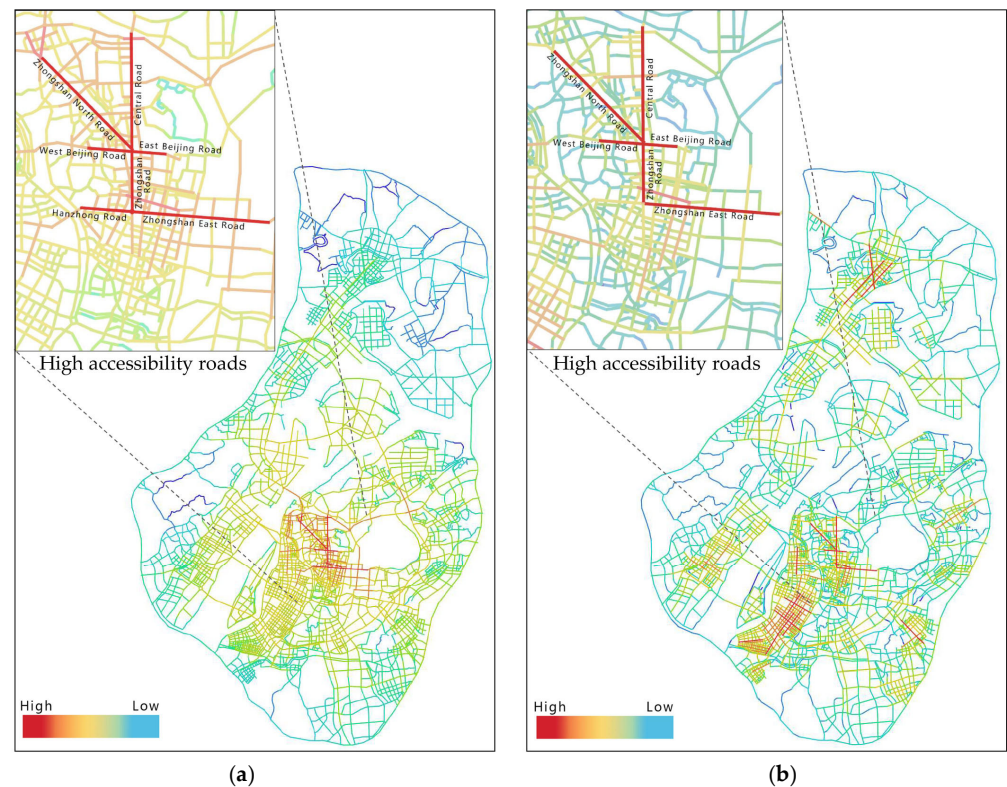
Figure 9. (a) Global integration analysis when R = n , red roads are roads with high accessibility; (b) Local integration analysis when R = 3 , red indicates roads with high accessibility.
