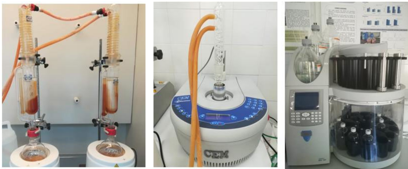
Figure 2. Comparisons of classical extraction methodologies (Soxhlet) with new alternatives: microwave-assisted extraction (MAE) or accelerated solvent extraction (ASE) systems (from left to right). Source ICSURO.
