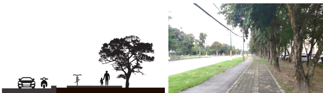
Figure 4. The cross-section of walkway No. 1: walkway with sparse trees on one side.
