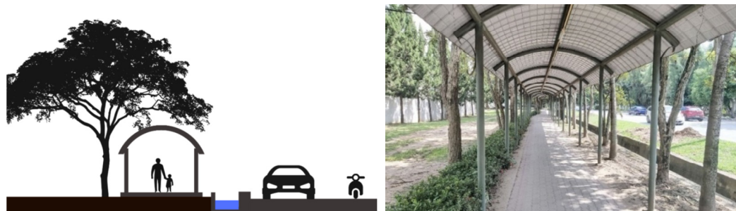
Figure 7. The cross-section of walkway No. 4: open-sided covered walkway with sparse trees.
