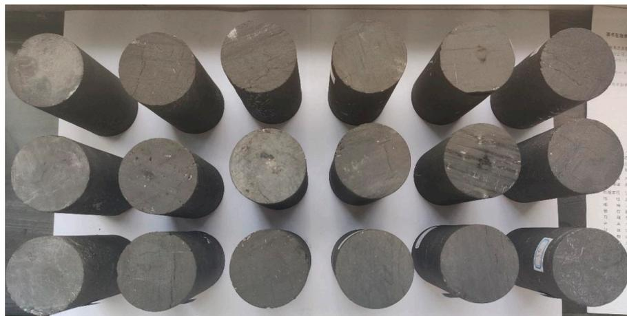
**Figure 2.** Partial coal specimens.
