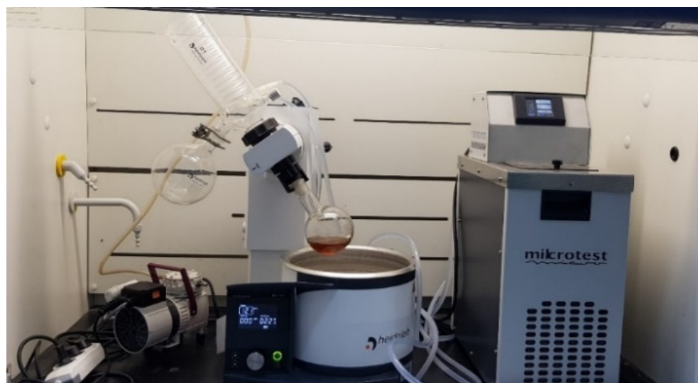
Figure 5. The evaporator and heater that were used in the experiments [34].
