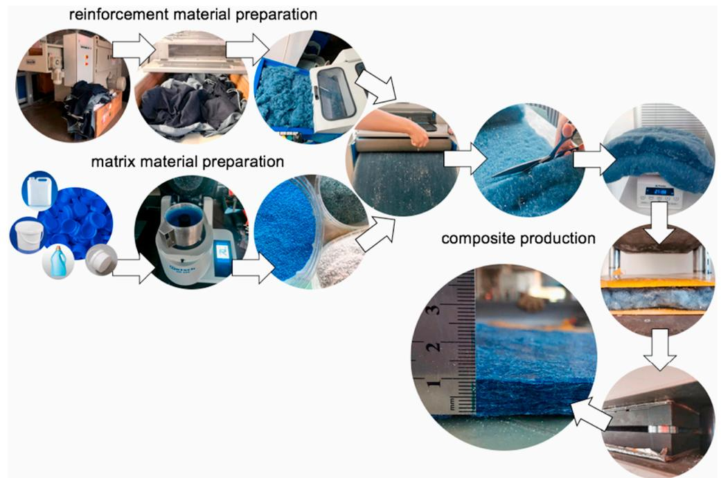
**Figure 23.** Fabrication of a composite insulation material using waste cotton and PP/PE fibers [166].
