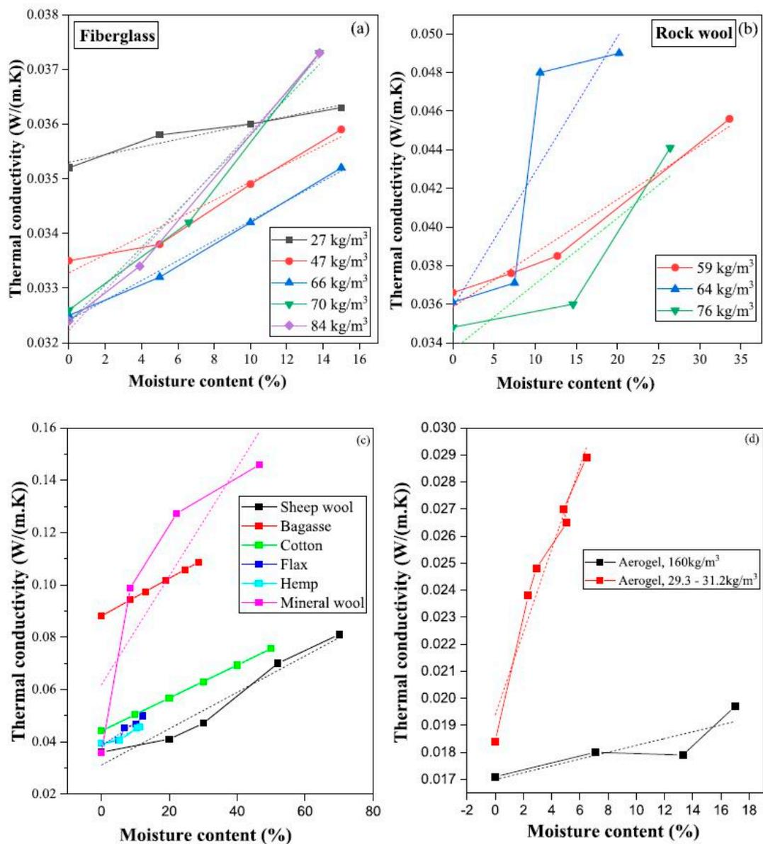
**Figure 30.** Effect of moisture content on the thermal conductivity of various insulation materials and varying densities; (a) fiberglass; (b) rockwool; (c) natural materials; and (d) aerogels [25].
