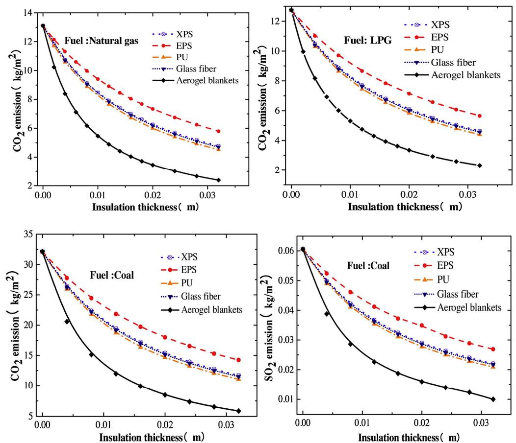
Figure 14. CO<sub>2</sub> and SO<sub>2</sub> emissions for various thicknesses of the insulation material [93].
