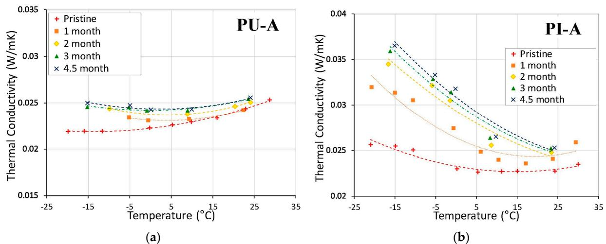
**Figure 31.** Effect of aging on thermal conductivity under various temperatures; (a) effect on polyurethane; and (b) effect on polyisocyanurate [213].
