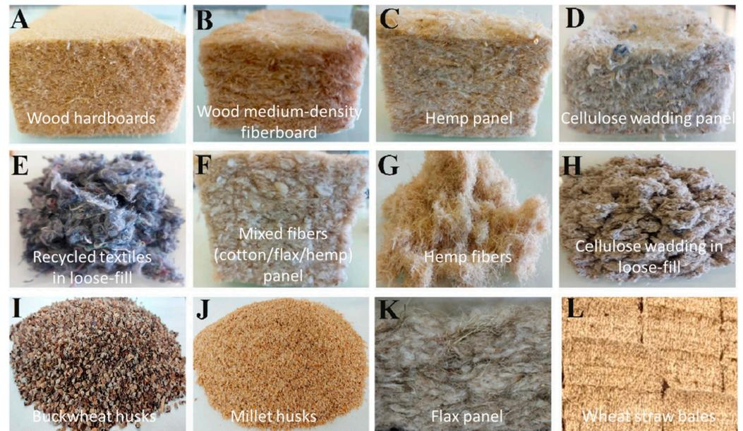
**Figure 18.** Various bio-mass-based sustainable materials for thermal insulation; (A) wood hardboards; (B) medium density wooden fiberboard; (C) Hemp panel; (D) Cellulose panels in compacted form; (E) recycled textile fibers; (F) mixture of cotton, flax and hemp fibers; (G) hemp fibers; (H) cellulose fiber in loose fill; (I) wheat husk; (J) millet husk; (K) flax panel; and (L)wheat straw bales [118].
