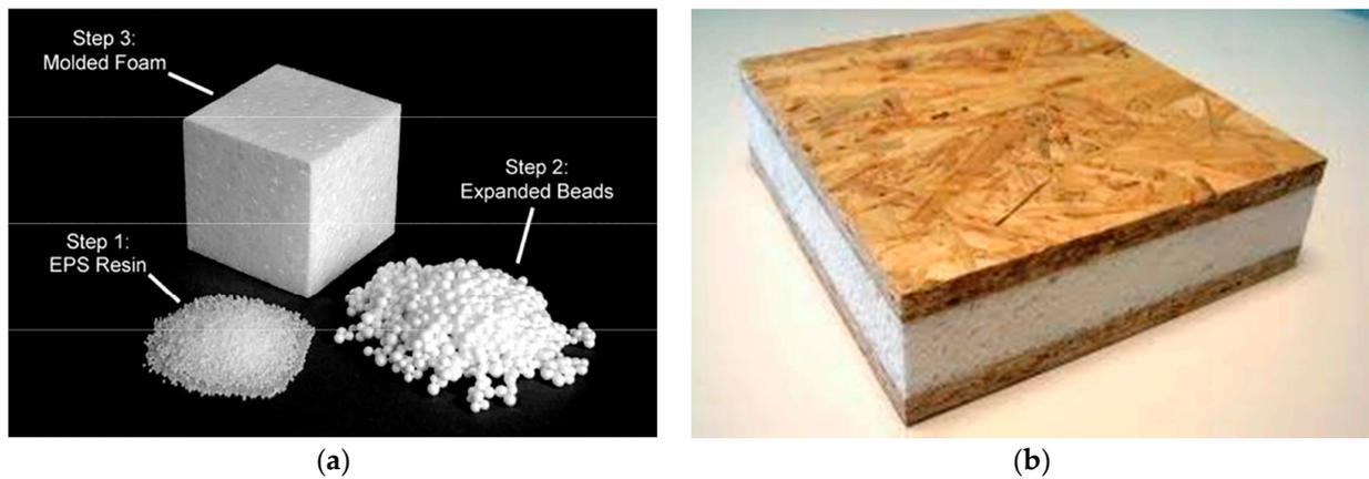
**Figure 8.** (a) Fabrication process of EPS; (b) application of EPS for structural panel insulation [57,76].
