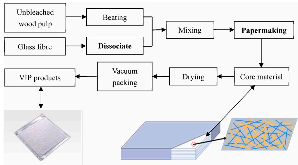
**Figure 24.** Composite vacuum insulation panels with wood pulp and glass fiber as a core material [168].
