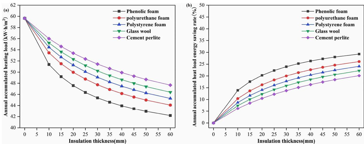
**Figure 26.** Effect of insulation thickness on heating load demand and annual energy saving; (a) reduction in heating load demand; and (b) increase in energy saving [172].
