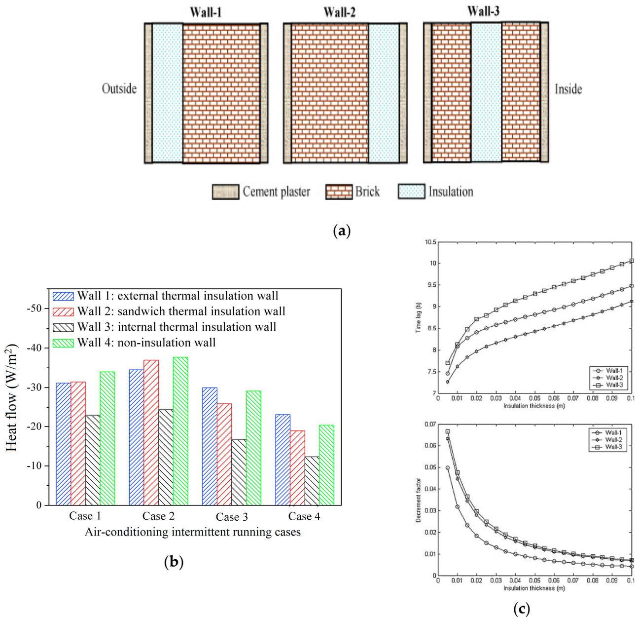
**Figure 27.** (a) Various insulation layer configurations; (b) variation in R-value corresponding to adopting insulation on the inside and outside of the panel; and (c) effect of insulation on time lag and decrement factor [184,185].
