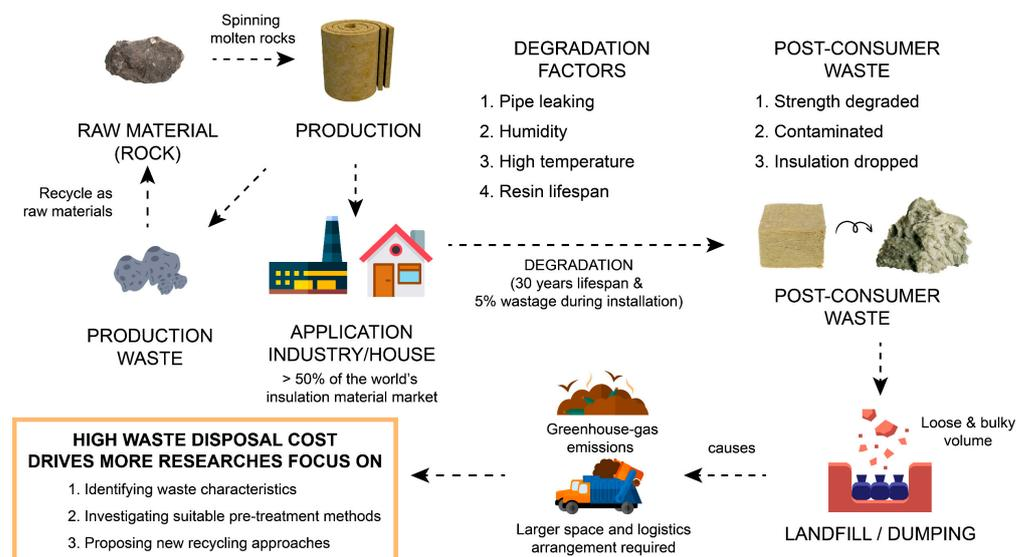
Figure 6. Production process of the mineral wool and its post-consumption recycling [32].
