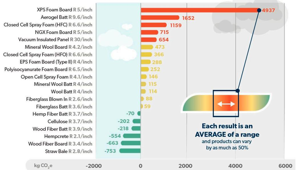
Figure 13. Material carbon emission for various commonly used insulation materials [92].
