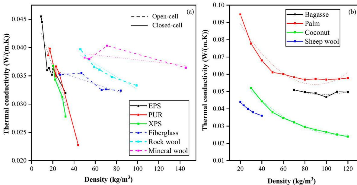
**Figure 29.** Variation in thermal conductivity with varying density for various insulation materials; (a) conventional materials used for insulation; and (b) natural fibrous materials [25].
