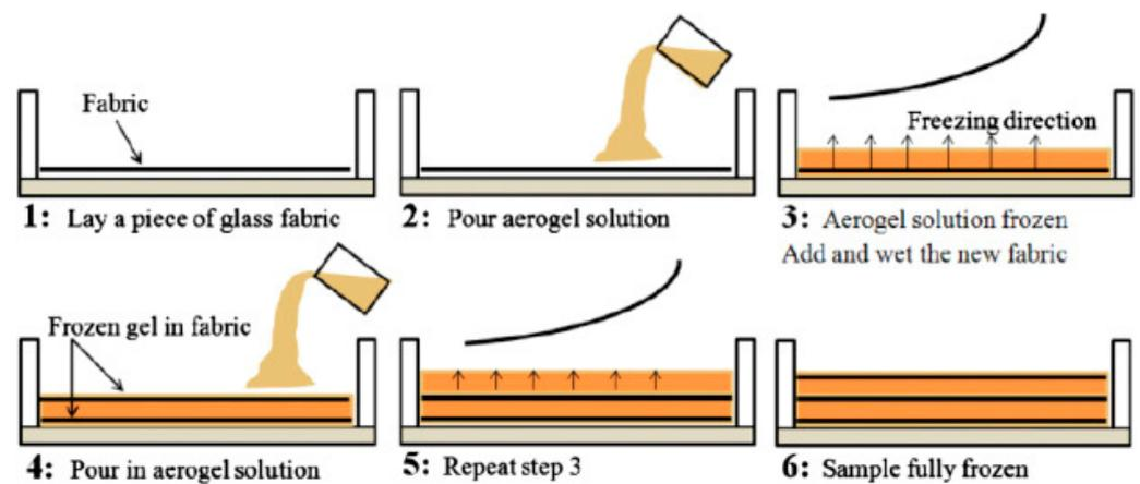
Figure 20. Fabrication process of glass fiber reinforced aerogel composites [142].
