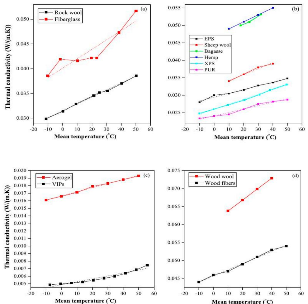
**Figure 28.** Effect of temperature variation on the thermal conductivity of various commonly used insulation materials: (a) inorganic materials; (b) organic materials; (c) advanced materials; and (d) combined materials [25].
