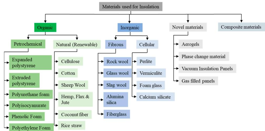
Figure 4. Classification of materials used for insulation.
