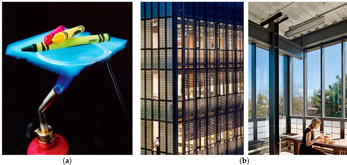
**Figure 19.** (a) Silica-based aerogel and (b) application range of aerogel in the building sector [123,133].
