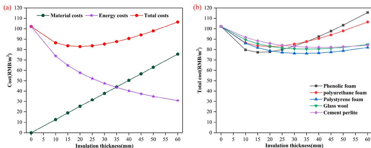
**Figure 25.** Comparison of insulation layer thickness and cost of various insulation materials; (a) comparison of insulation material cost with energy cost with varying insulation thickness; and (b) variations in total cost for various material with varying insulation thickness [172].
