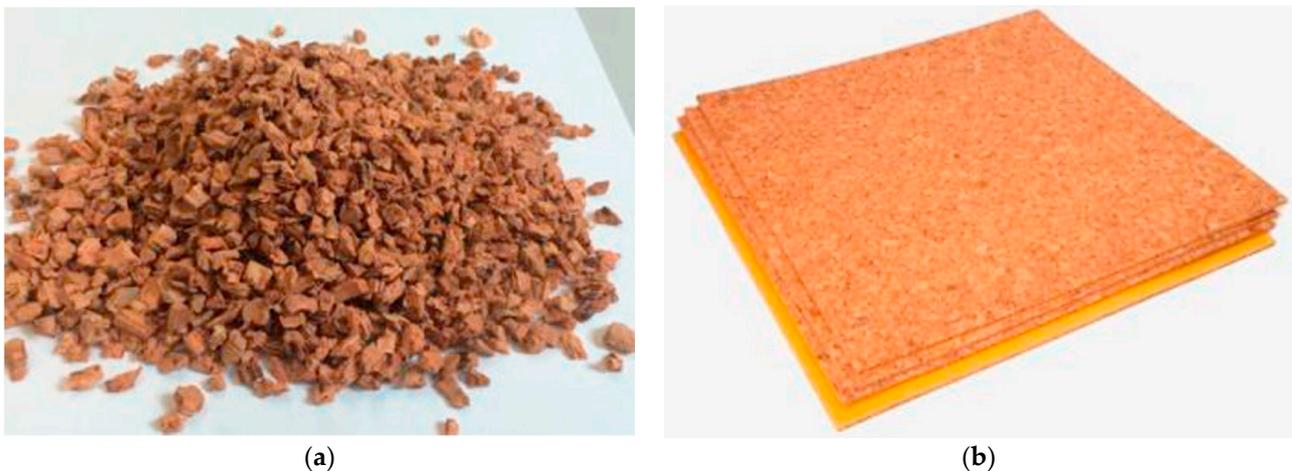
**Figure 17.** (a) Cork particles in natural form; and (b) application of cork panels for structure insulation [107].
