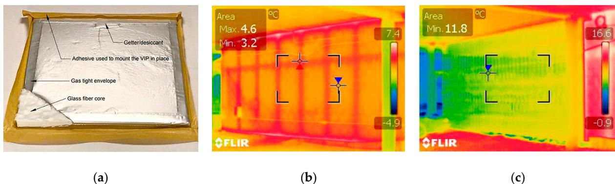
**Figure 22.** (a) Glass fiber core vacuum insulation panel; (b) thermal infrared imageries of the model before retrofitting with insulation; and (c) after retrofitting with insulation [157].
