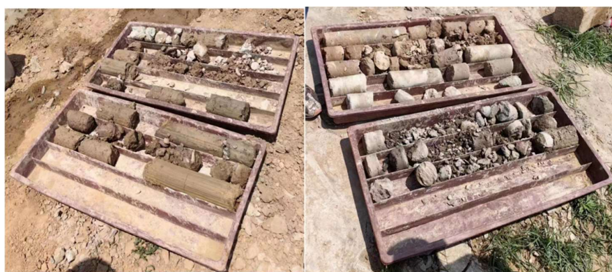
Figure 2. Coring of conventional deep mixing techniques.
