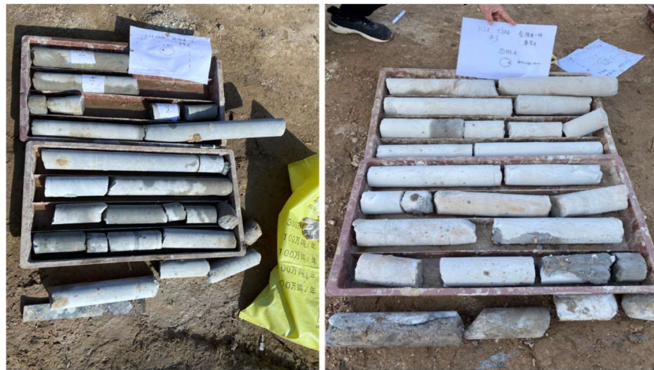
Figure 4. Coring of DMJ pile techniques.
