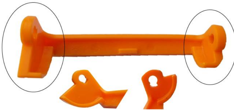
Figure S6. Floor nozzle brush locking cap. The circles at the sides of the figure indicate the locations of the enlarged partial overviews at the bottom of the figure.
