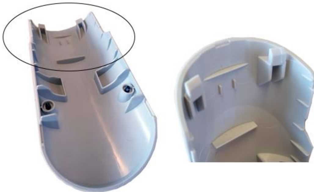
Figure S8. Floor nozzle cable cover. The circle at the top of the figure indicates the location of the enlarged partial overview at the right of the figure.
