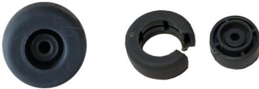
Figure S1. Floor nozzle wheel intact (left) and with separate tyre and hub (right).
