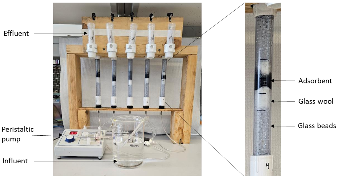
Figure S1: Column apparatus set-up
