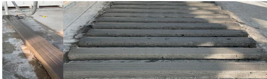
**Figure 23.** Stable extrusion filaments of a rectangular nozzle in the N-path.
