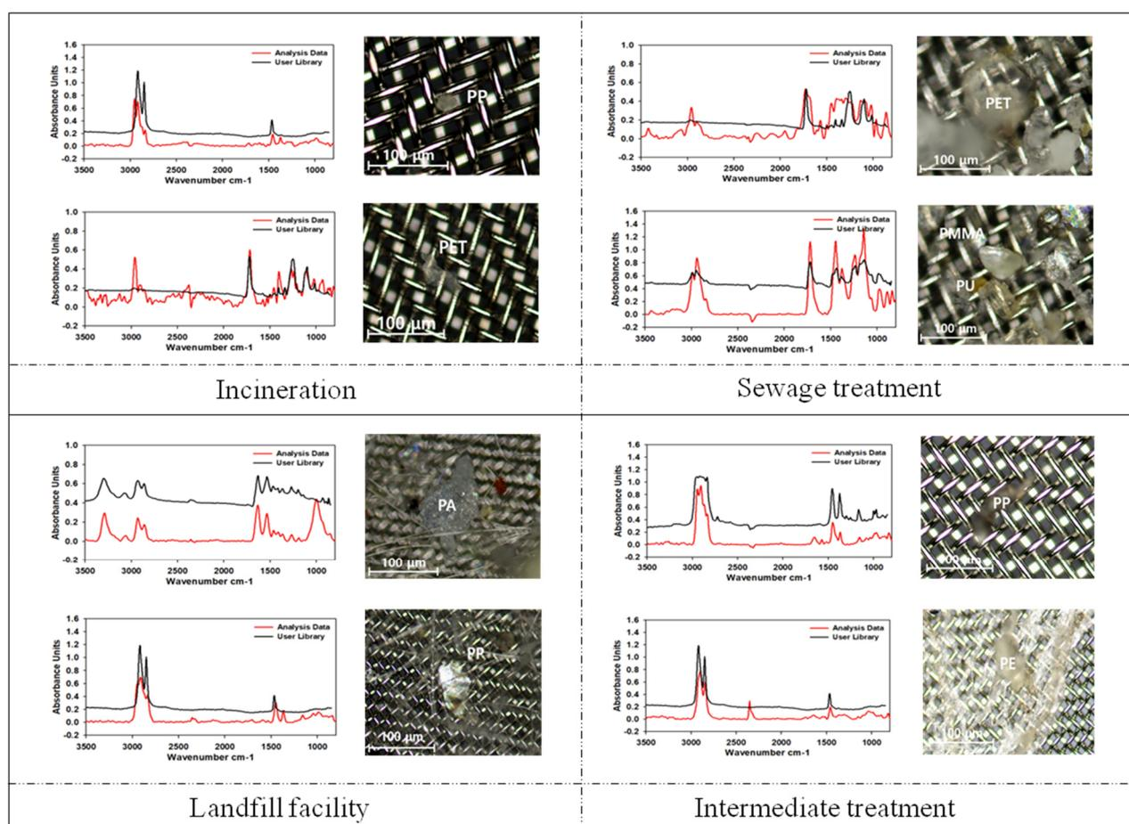
**Figure 3.** FT-IR spectrum and image of MPs.
