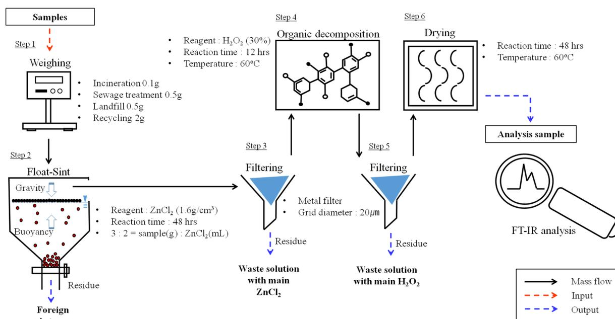
**Figure 2.** Schematic flow diagram for preparing samples for FT-IR analysis.
