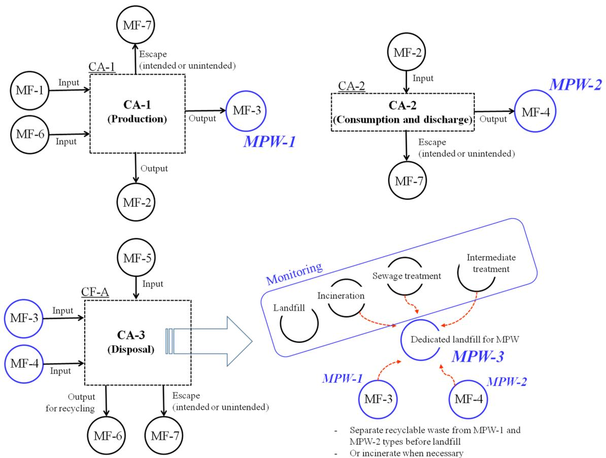
**Figure 4.** Flows of MPW-1, MPW-2, and MPW-3 in each part of the circular system. The red dotted arrows indicate “landfilled”.
