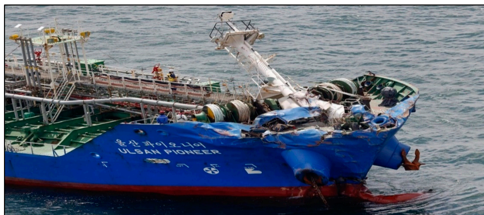
Figure 8. The bulbous bow of Ulsan Pioneer after collision (adapted from [65]).
