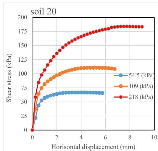
Figure 18. Direct shear test result for natural (untreated) gypseous soil 20.
