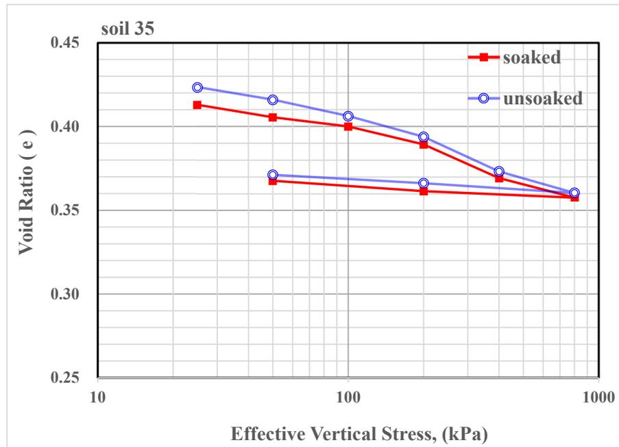
**Figure A2.** Double oedometer test result for the 2.5% geopolymer-treated gypseous soil 35.
