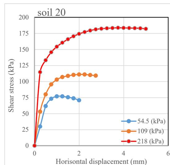
**Figure 21.** Direct shear test result for 2.5% geopolymer-treated gypseous soil 20.
