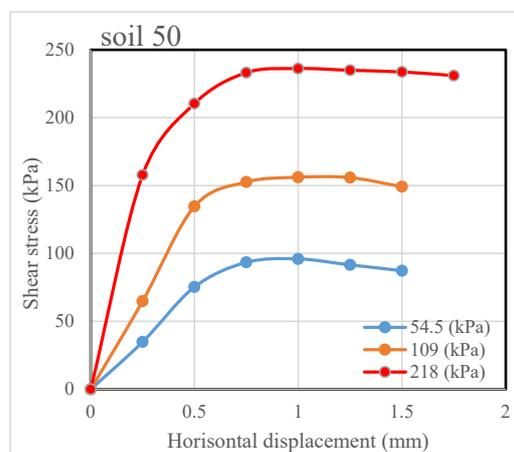
Figure 27. Direct shear test result for the 2.5% geopolymer-treated gypseous soil 50.
