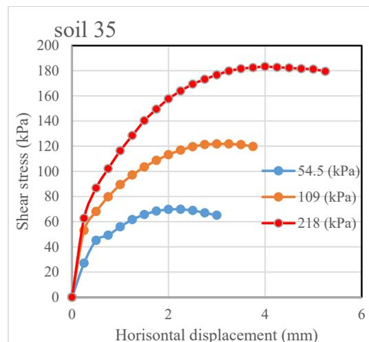
Figure 19. Direct shear test result for natural (untreated) gypseous soil 35.
