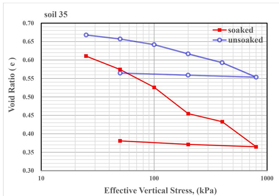
Figure 8. Double oedometer test result for the natural (untreated) gypseous soil 35.
