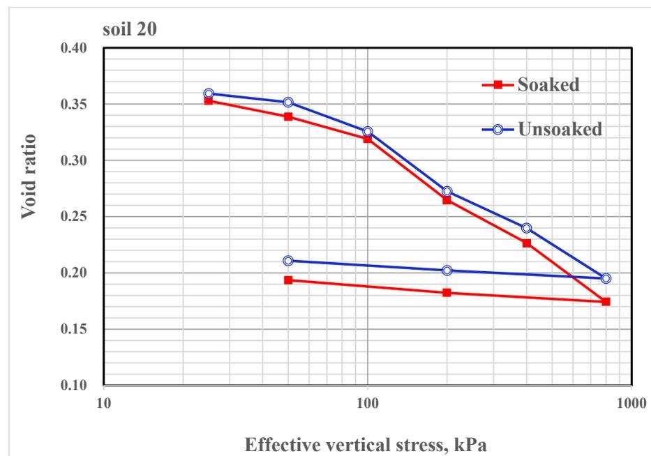
Figure 12. Double oedometer test result for the 2.5% geopolymer-treated gypseous soil 20.
