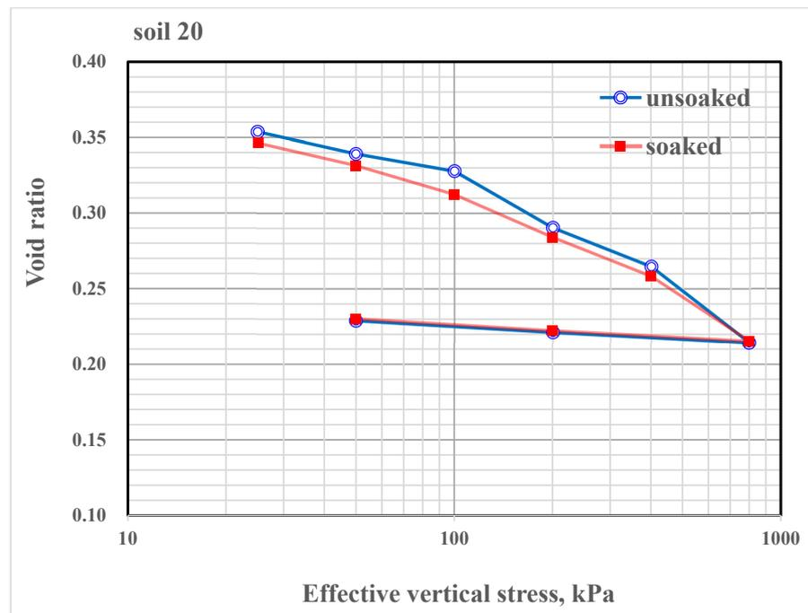
Figure 13. Double oedometer test result for the 5% geopolymer-treated gypseous soil 20.
