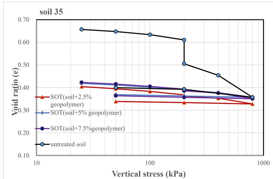
**Figure A1.** Single oedometer test result for the geopolymer-treated gypseous soil 35.
