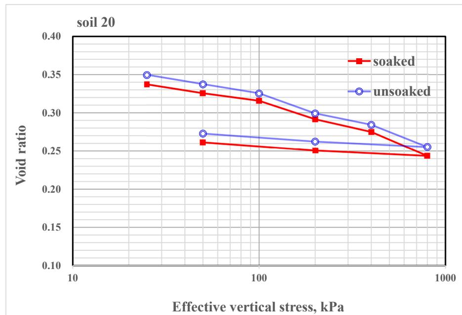
Figure 14. Double oedometer test result for the 7.5% geopolymer-treated gypseous soil 20.
