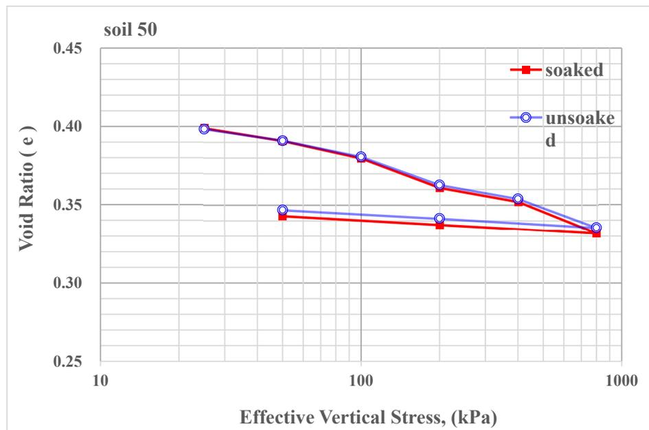
Figure A6. Double oedometer test result for the 2.5% geopolymer-treated gypseous soil 50.
