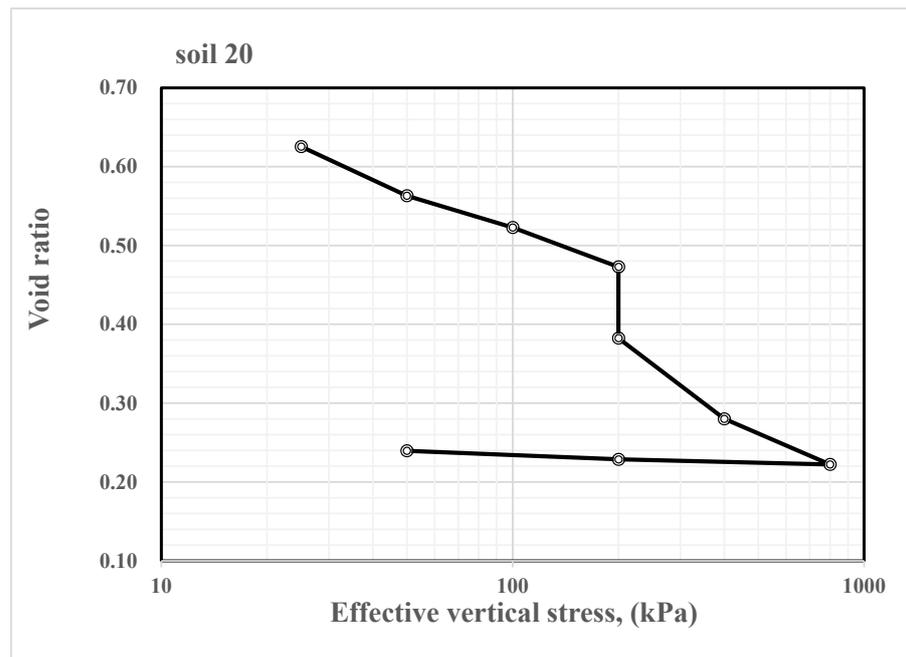
Figure 5. Single oedometer test result for the natural (untreated) gypseous soil 20.
