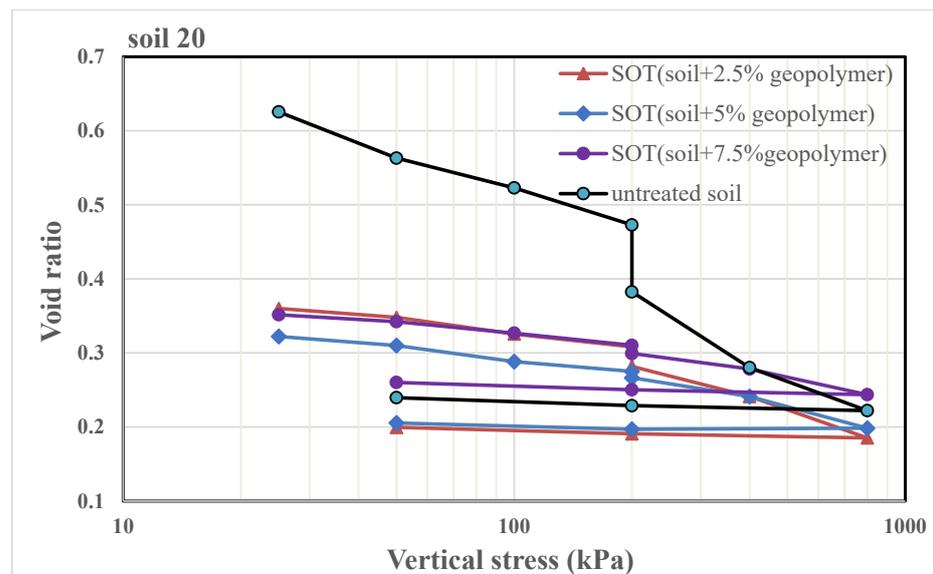
Figure 11. Single oedometer test result for the geopolymer-treated gypseous soil 20.
