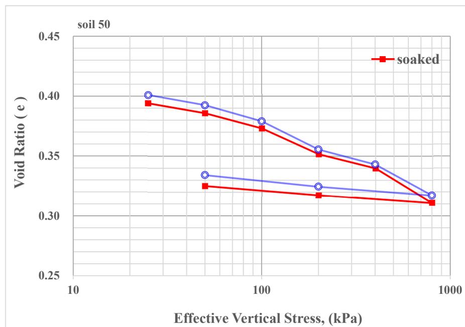
Figure A7. Double oedometer test result for the 5% geopolymer-treated gypseous soil 50.
