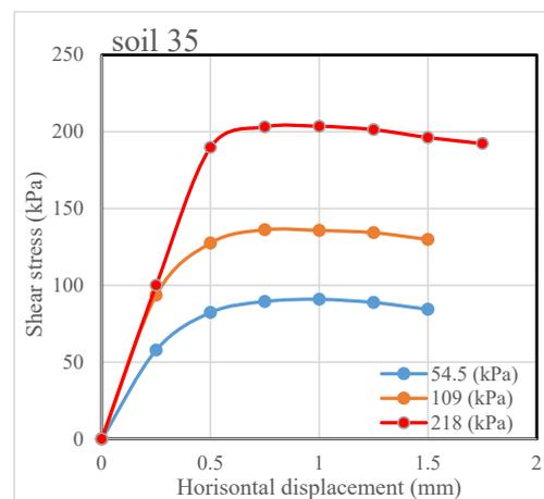
Figure 24. Direct shear test result for the 2.5% geopolymer-treated gypseous soil 35.
