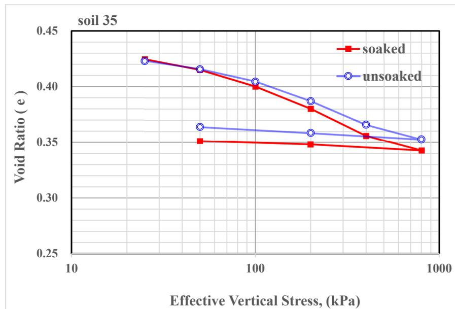
Figure A4. Double oedometer test result for the 7.5% geopolymer-treated gypseous soil 35.
