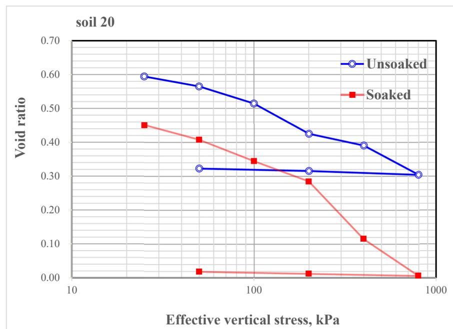
Figure 6. Double oedometer test result for natural (untreated) gypseous soil 20.
