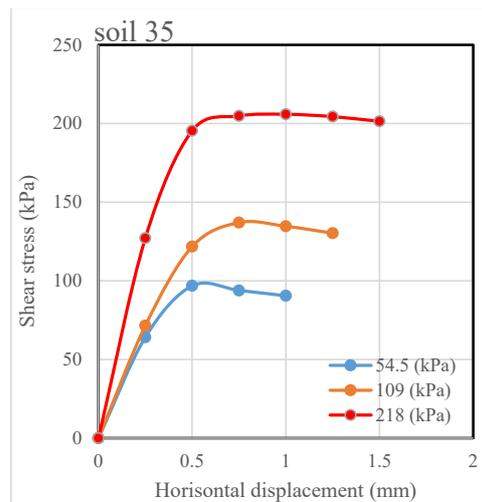
Figure 25. Direct shear test result for the 5% geopolymer-treated gypseous soil 35.
