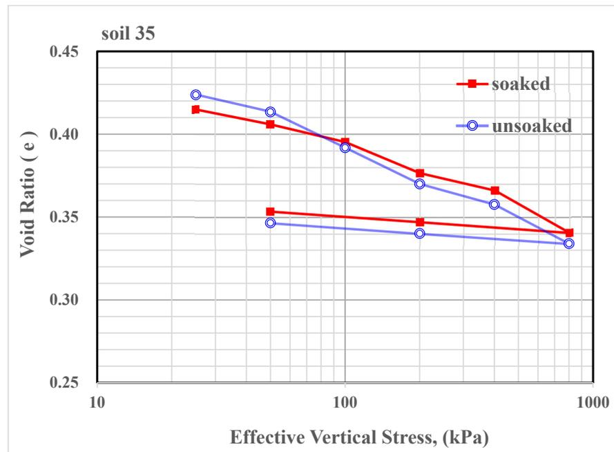
Figure A3. Double oedometer test result for the 5% geopolymer-treated gypseous soil 35.
