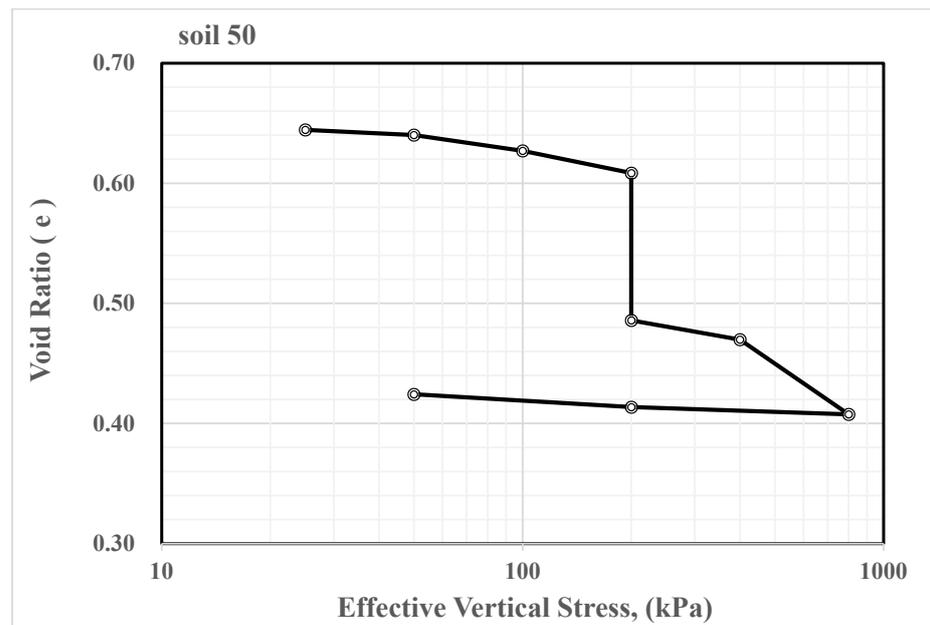
Figure 9. Single oedometer test result for the natural (untreated) gypseous soil 50.
