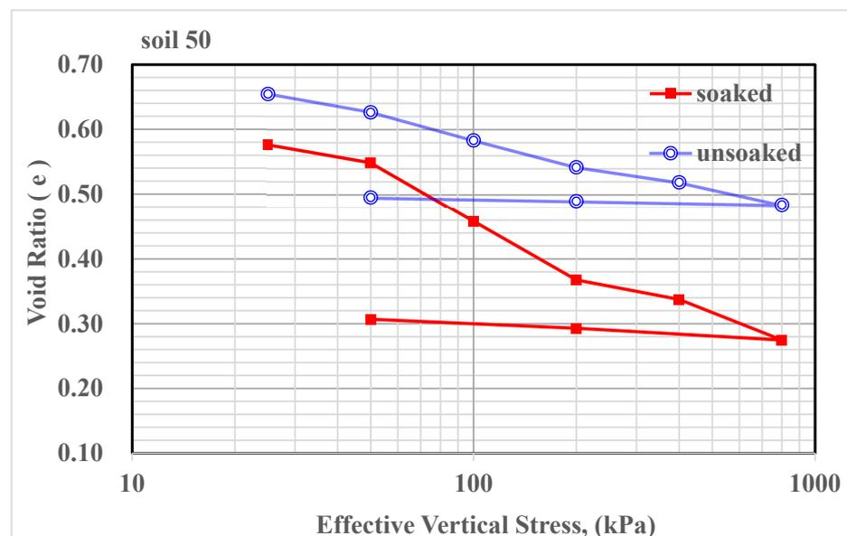
Figure 10. Double oedometer test result for the natural (untreated) gypseous soil 50.
