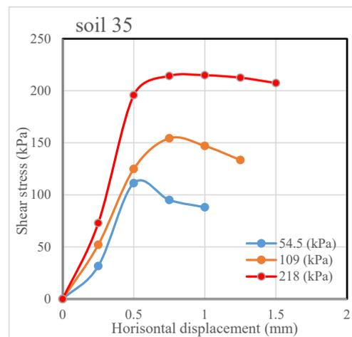
Figure 26. Direct shear test result for the 7.5% geopolymer-treated gypseous soil 35.
