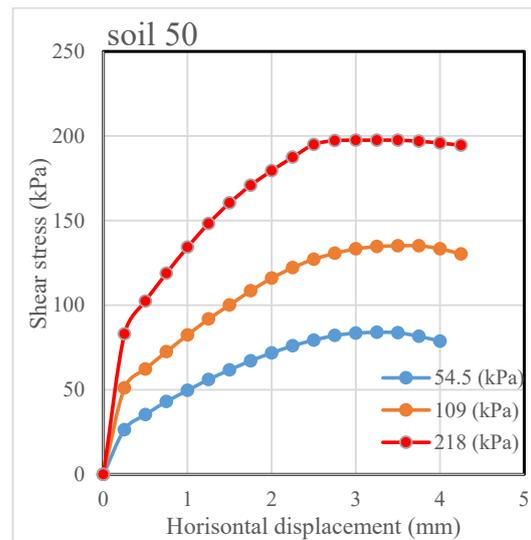
**Figure 20.** Direct shear test result for natural (untreated) gypseous soil 50.
