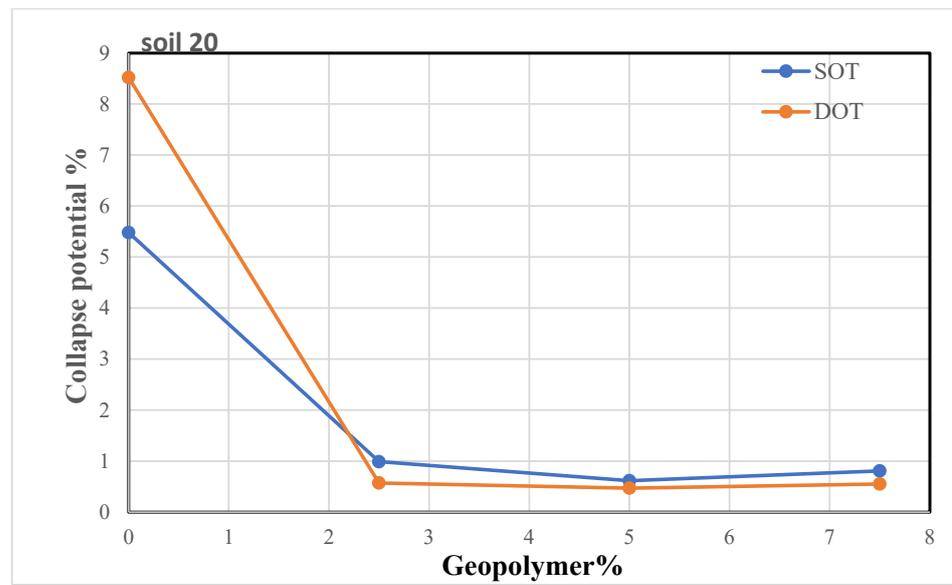
**Figure 15.** Effect of geopolymer concentration on single and double oedometer test collapse potential for soil 20.
