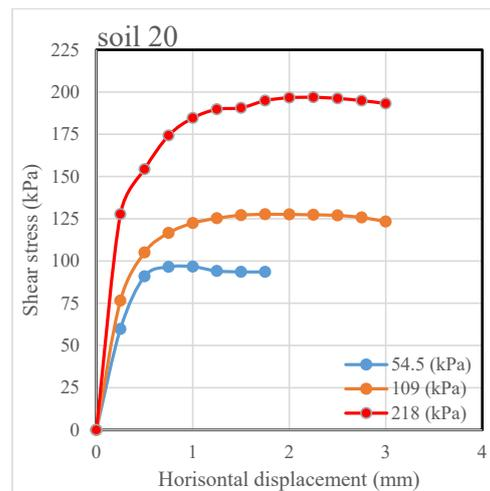
Figure 22. Direct shear test result for the 5% geopolymer-treated gypseous soil 20.
