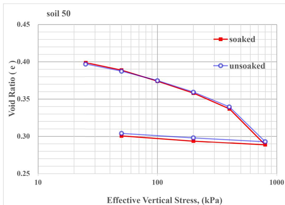
Figure A8. Double oedometer test result for the 7.5% geopolymer-treated gypseous soil 50.
