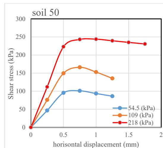
**Figure 29.** Direct shear test result for the 7.5% geopolymer-treated gypseous soil 50.
