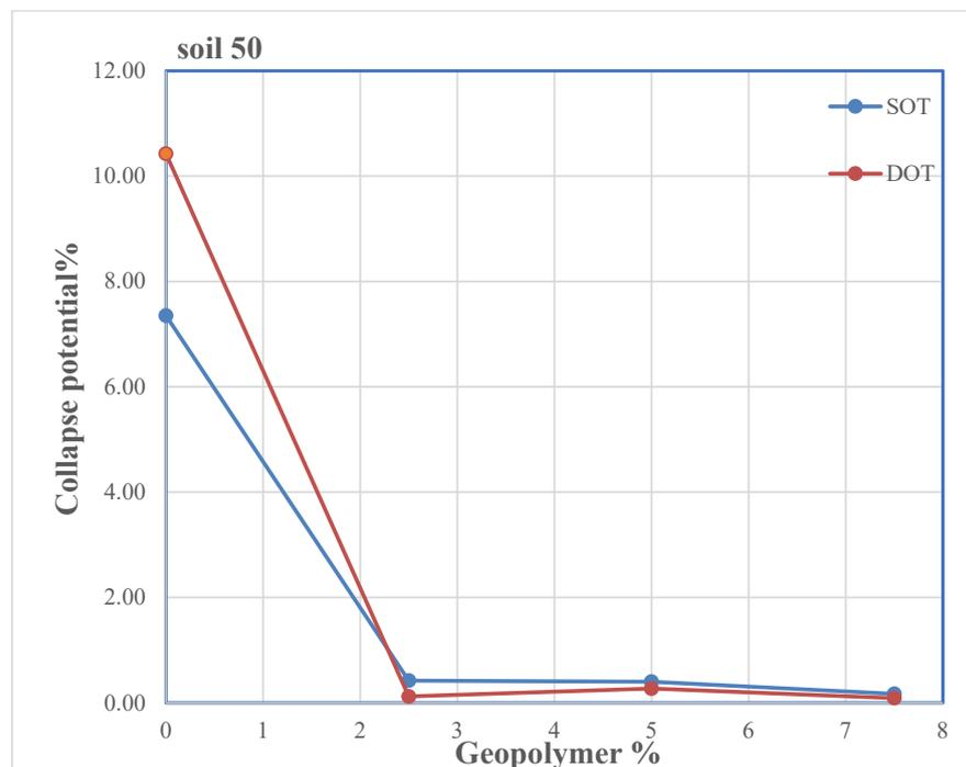
**Figure 17.** Effect of geopolymer concentration on single and double oedometer test collapse potential for soil 50.
