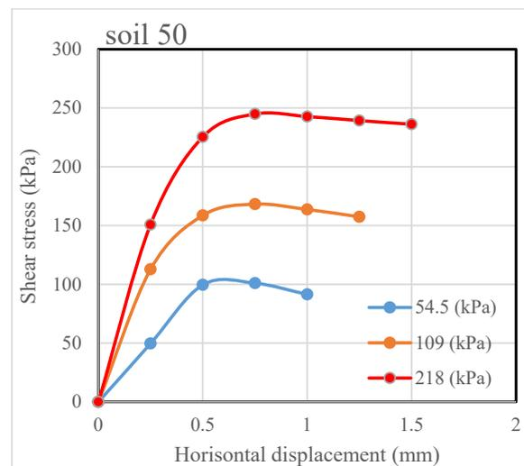
**Figure 28.** Direct shear test result for the 5% geopolymer-treated gypseous soil 50.
