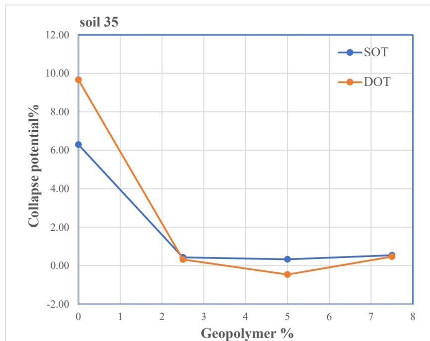
**Figure 16.** Effect of geopolymer concentration on single and double oedometer test collapse potential for soil 35.
