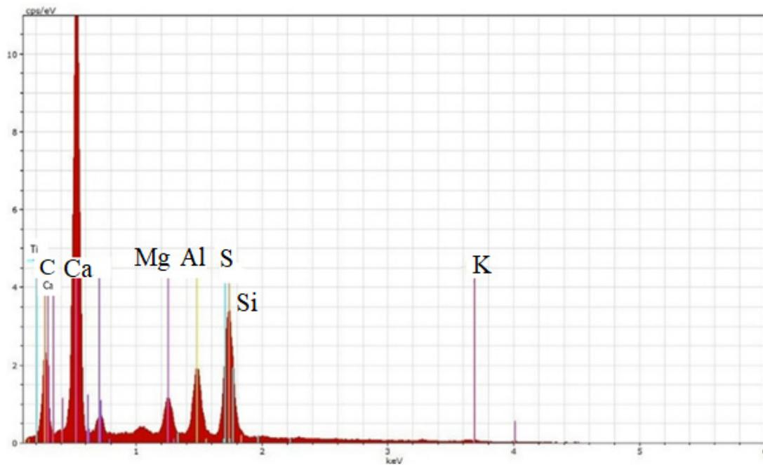
**Figure 3.** EDX spectrometry for the CCR.
