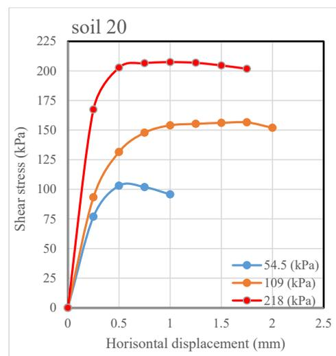
Figure 23. Direct shear test result for the 7.5% geopolymer-treated gypseous soil 20.
