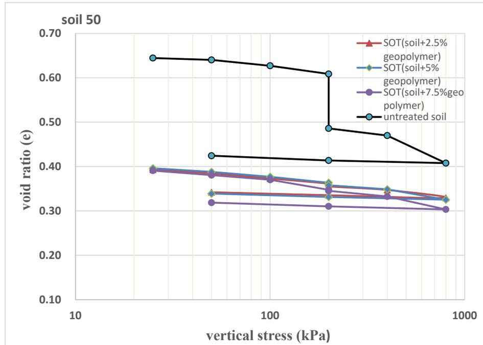
Figure A5. Single oedometer test result for the geopolymer-treated gypseous soil 50.
