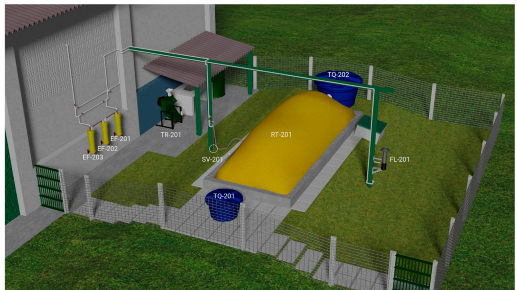
Figure 1. Low-cost pilot plant developed for biogas and biofertilizer production from food waste on experimental biorefinery of organic solid waste. TR-201: food grinding machine; TQ-201: feeding tank; RT-201: pilot biodigester; TQ-202: storing biofertilizer tank; SV-201: safety valve; FL-201: flare; EF-201: filter 1; EF-202: filter 2; EF-203: filter 3. Source: [28].
