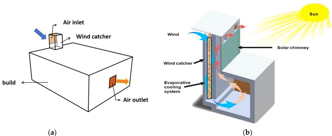
**Figure 7.** Schematic diagram of building ventilation assisted by a unilateral wind catcher [64]: (a) single-sided wind catcher; (b) wind catcher combined with solar chimney [75].
