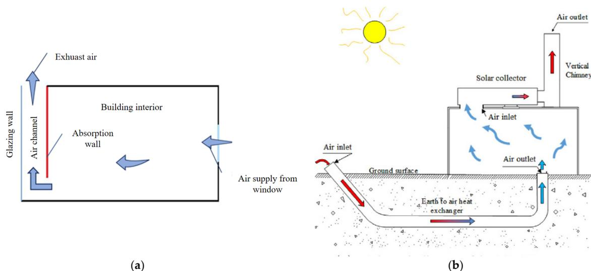
**Figure 9.** Schematic diagram of solar chimney-assisted building ventilation: (a) solar chimney [93]; (b) solar chimney combined with an EAHE [94].
