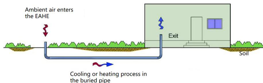
**Figure 8.** Schematic diagram of building ventilation assisted by an EAHE [85].
