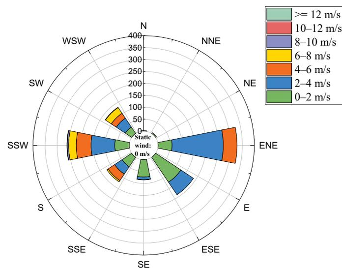
**Figure 3.** Winter ambient wind speed distribution measurement in the Ngari Region of Tibet (4300 m above sea level).
