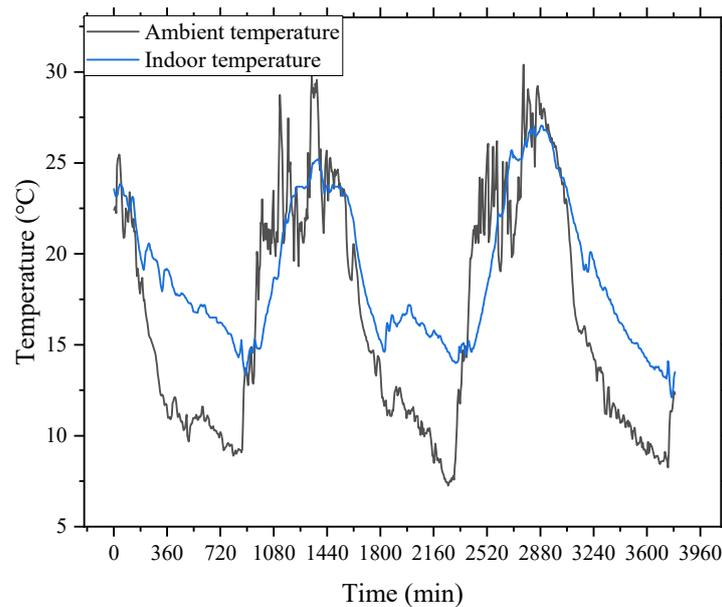
**Figure 5.** Comparison of indoor and outdoor temperatures in a lightweight underground building in the Ngari region of Tibet during summer.
