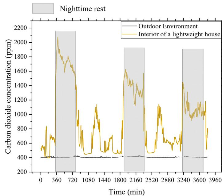
**Figure 6.** Comparison of indoor and outdoor carbon dioxide levels in a lightweight underground building in the Ngari region of Tibet during summer.
