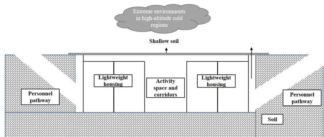
**Figure 4.** Schematic diagram of the layout of underground lightweight prefabricated houses in cold plateau regions.
