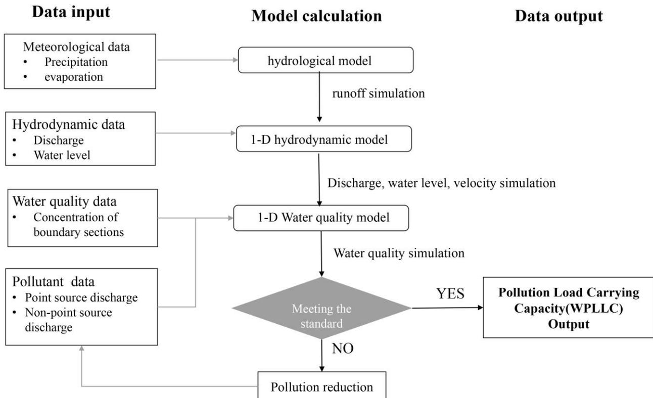
**Figure 3.** Framework of pollution load carrying capacity calculation by 1-D mathematical modeling simulation.
