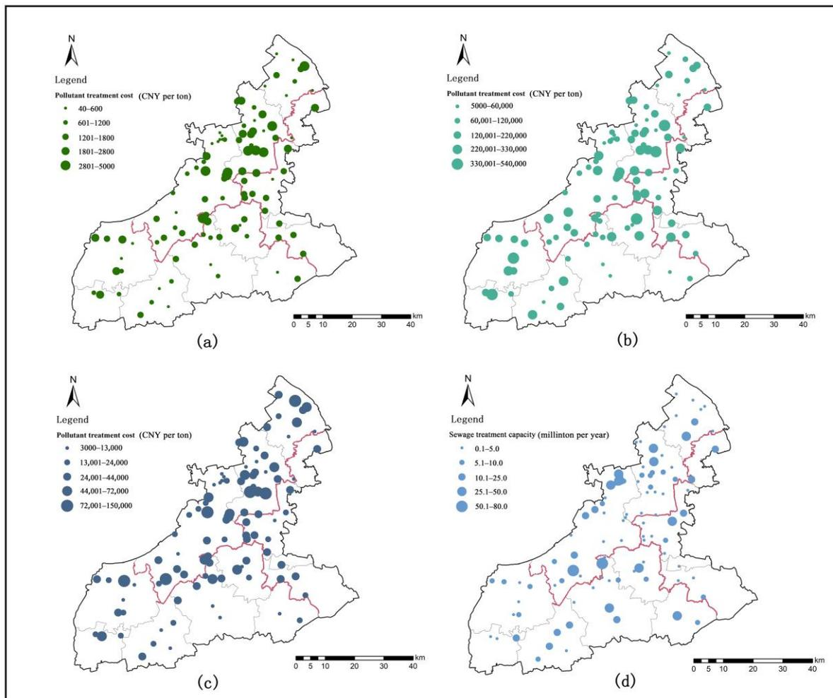
**Figure 8.** The treatment cost per unit for pollutants: (a) COD, (b) TP, (c) NH<sub>3</sub>-N, and (d) treatment capacity of the 98 sewage plants in TECS.
