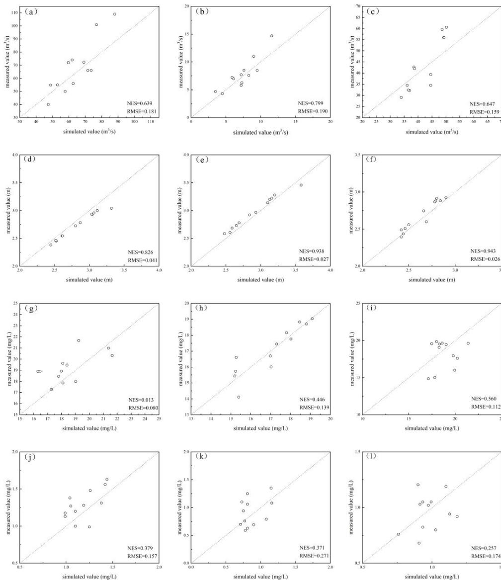
**Figure 2.** Comparison of measured and simulated results of established 1-D mathematical model. (a–c) refer to discharge at site 29, site 12, and Section 5, respectively; (d–f) refer to water level of site 29, site 12, and Section 5, respectively; (g–i) refer to the concentration of  $\text{NH}_3\text{-N}$  at site 29, site 12, and Section 5, respectively; (j–l) refer to concentration of TP at site 29, site 12 and site 5, respectively, in Figure 1.
