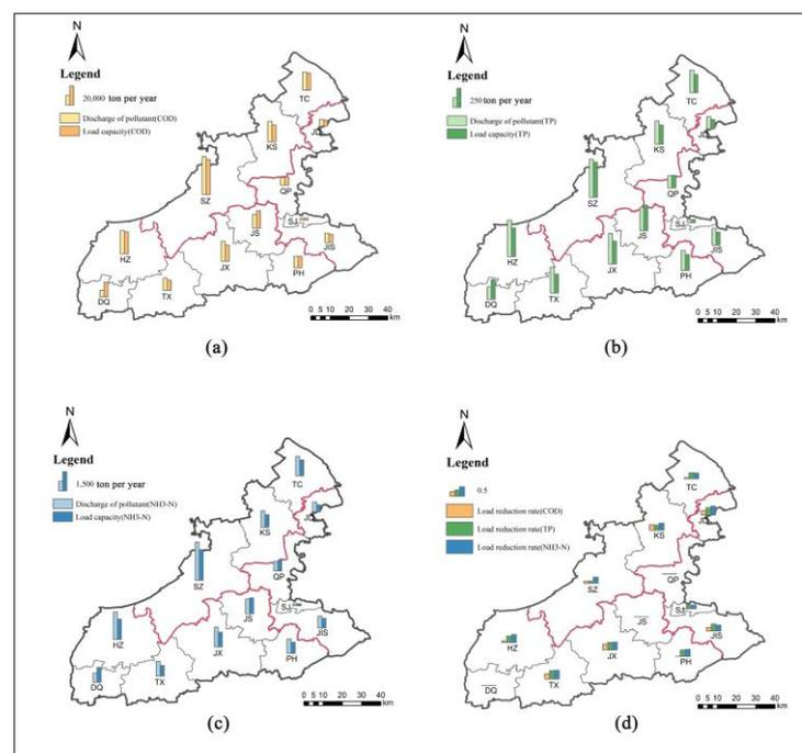
**Figure 7.** (a–c) Comparison of calculated load capacity and load discharging in 13 contributing administrative districts for COD (a), TP (b), and NH<sub>3</sub>-N (c); (d) distribution of calculated load reduction rates for pollutants COD, TP, and NH<sub>3</sub>-N in 13 contributing administrative districts.
