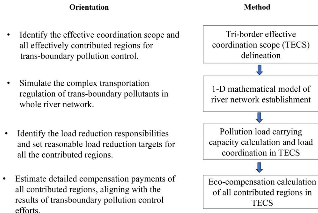
**Figure 4.** Flow chart of methodological framework for trans-boundary pollution control of complex river network.
