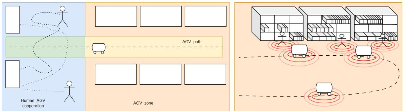
**Figure 4.** Examples of sharing space between humans and AGVs.
