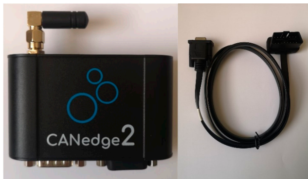
Figure 2. CANedge2 device used for bus data collection.
