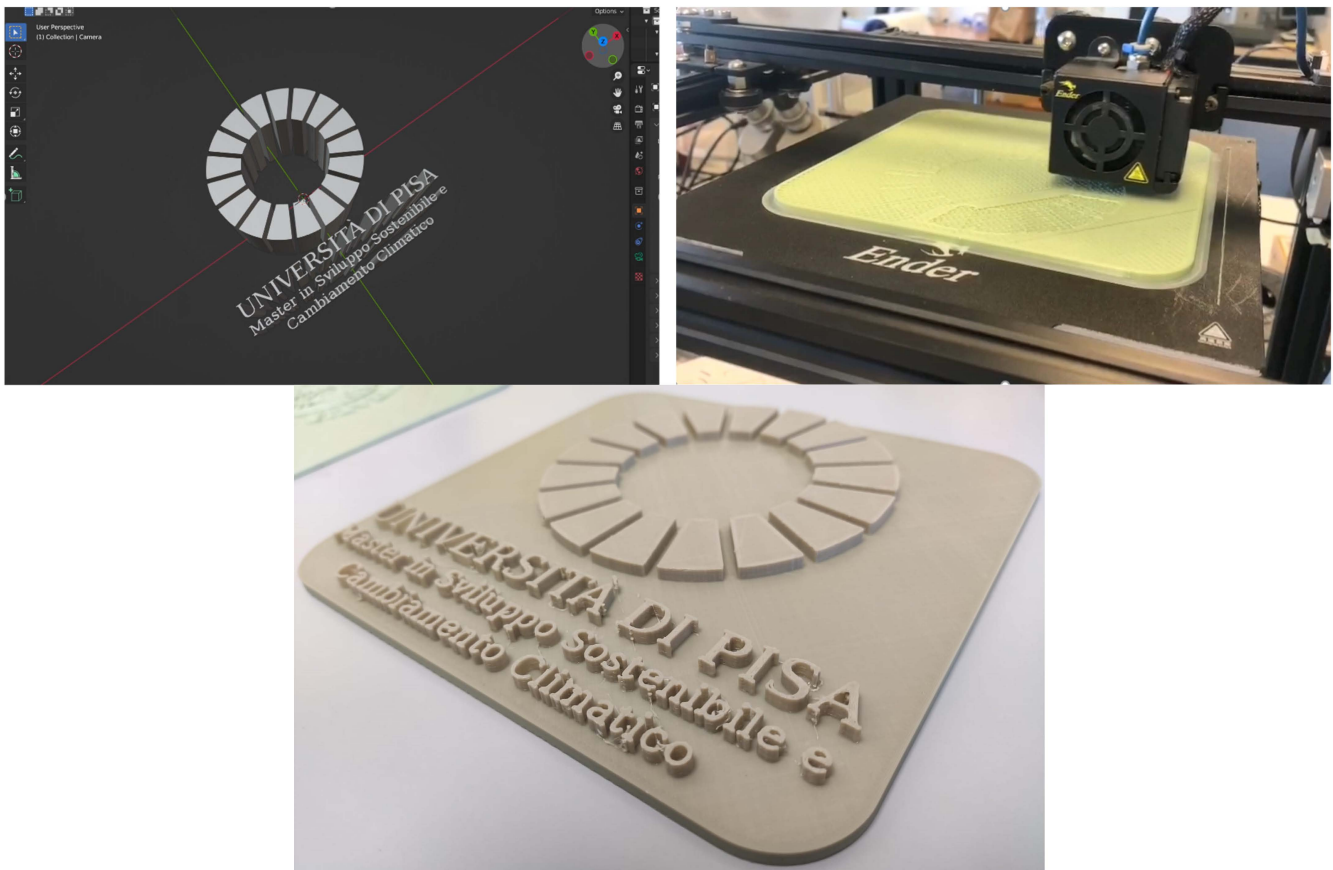
Figure 5. Digital project, realization, and the final product of the logo of the postgraduate master's course on Sustainable Development and Climate Change at the University of Pisa, produced by Working Group 3 with recycled plastic filaments.
