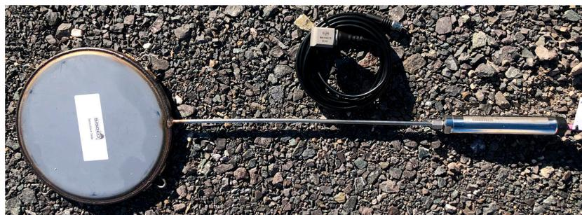
Figure 3. Pressure transducer Sisgeo L141 [24].
