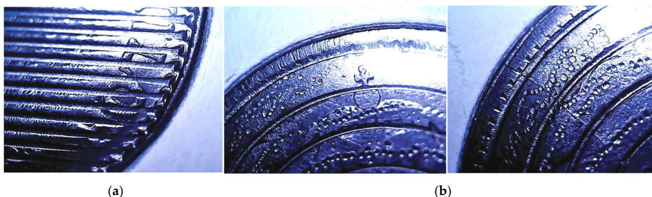
Figure 18. The concentric circles and fine parallel lines pattern canceled coin: (a) the unaffected obverse fine lines die, (b) the circled reverse die, affected by the initial fine flash line on edge and a radial die crack.
