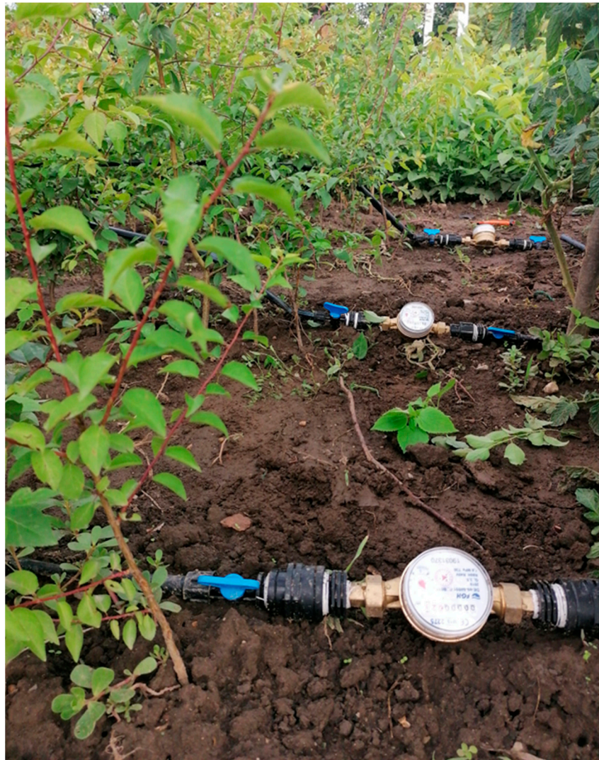
Figure 2. Irrigation control system in the nursery for measuring the amount of water used.
