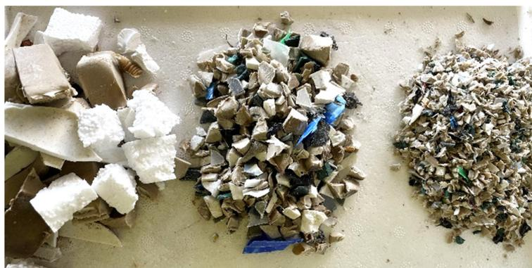
**Figure 2.** MWP feedstocks of three different sizes: 5 mm, 25 mm, and 45 mm.
