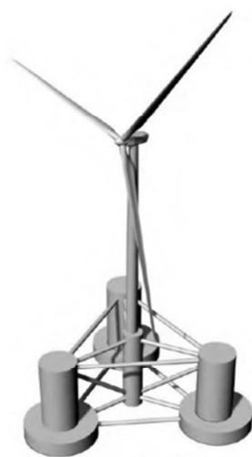
**Figure 1.** Semi-submersible wind turbine.
