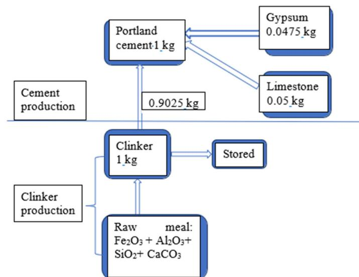
**Figure 1.** Material flow diagram for the production of 1 kg of Portland cement (adapted from the Ecoinvent database).
