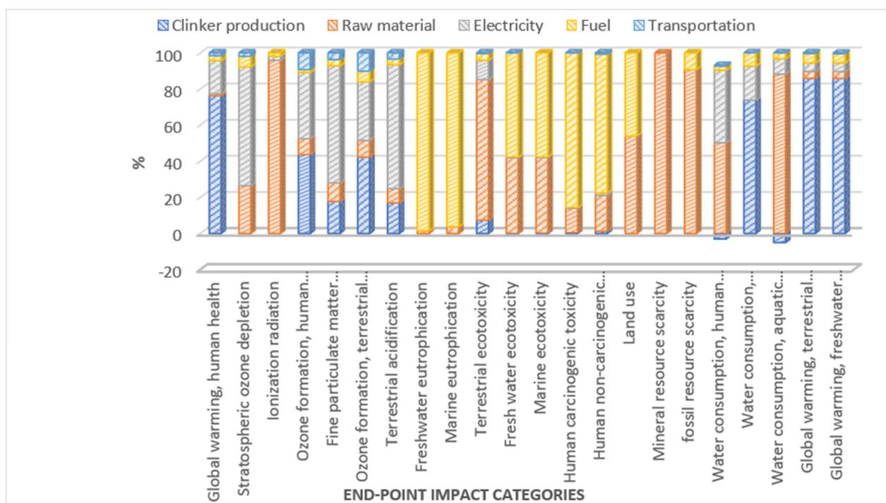
**Figure 8.** Contribution of five production processes to impact categories (end-point).
