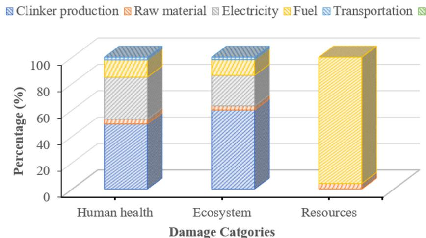
Figure 9. Contribution of five production processes to damage categories.
