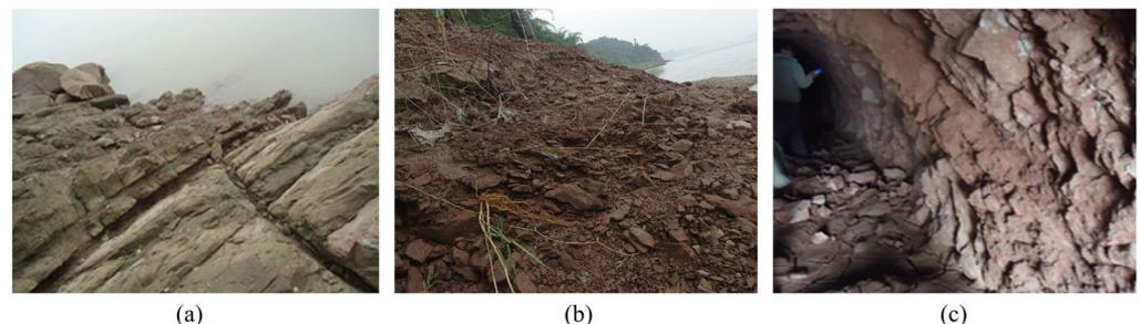
**Figure 2.** Bedrock samples from Xiaonanhai site: (a) silty claystone; (b) clayey siltstone; (c) feldspathic lithic sandstone.
