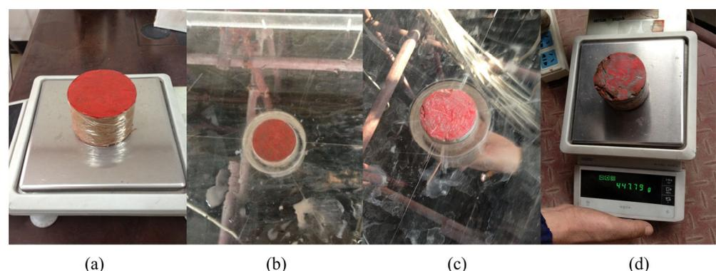
**Figure 5.** Bedrock incipient scour test sample conditions: (a) Weighing before the test; (b) Placing it in the top sample device before releasing water; (c) Observing scouring during the test; (d) Weighing the sample after removing it from the test.
