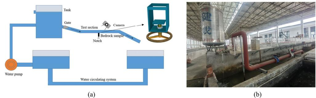
**Figure 3.** Illustration of the flume used to conduct bed erosion experiments. (a) Model schematic diagram; (b) Physical model.
