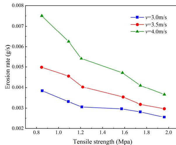
**Figure 9.** Plot of erosion rate versus tensile strength for different bed shear stresses.
