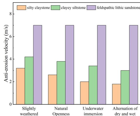
Figure 6. The corresponding anti-scour velocities of bedrock under various conditions.
