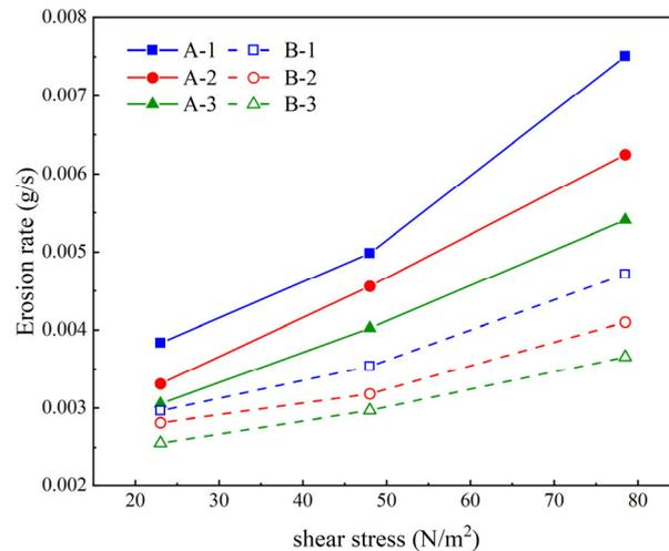
**Figure 8.** Plot of erosion rate versus bed shear stress for different bedrock samples.
