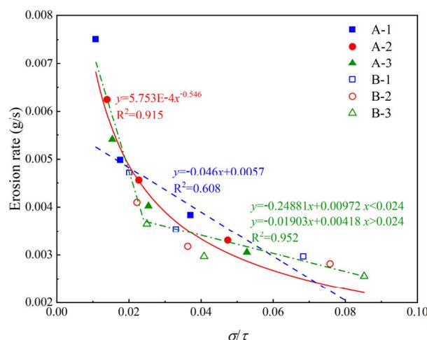
**Figure 10.** The erosion rate against the ratio of tensile strength to bed shear stress.
