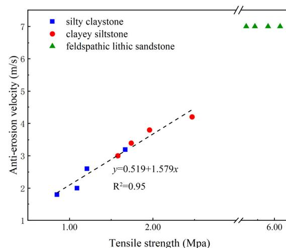
Figure 7. The relationship between the anti-scour velocity and tensile strength of the bedrock samples.
