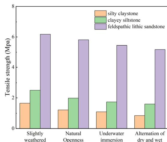
**Figure 4.** The tensile strengths corresponding to various types of bedrock samples.
