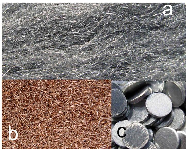
**Figure 2.** n-ZVM powder. (a) n- $Fe^0$ . (b) n- $Cu^0$ . (c) n- $Al^0$ .
