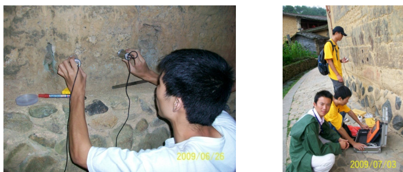
Figure 5. Ultrasonic testing heads and device.
