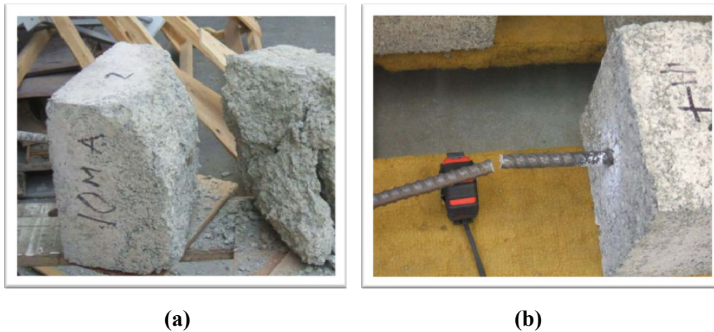
Figure 5. (a) 10M (#4) Sample after testing. (b) Bar failure in Pull Out test.
