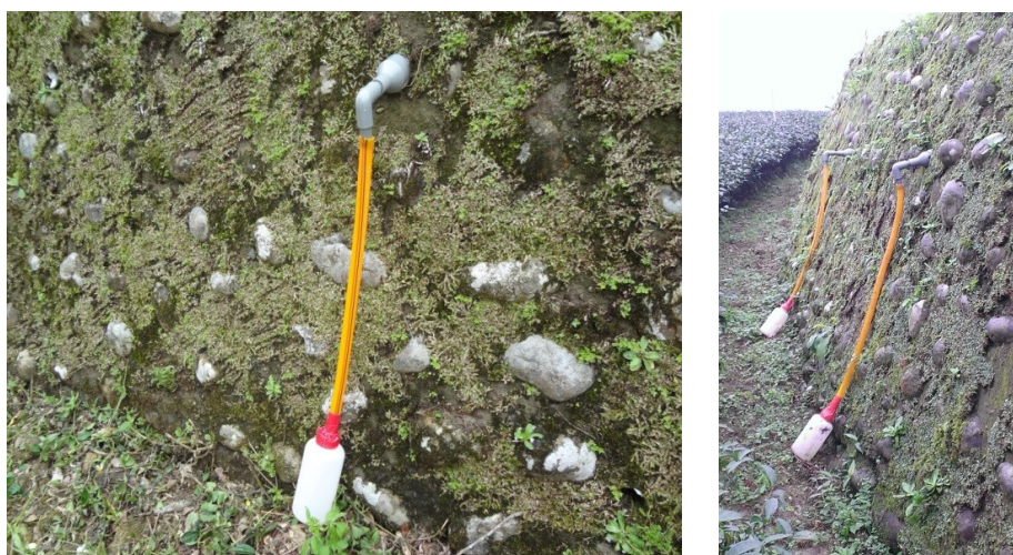
Figure 2. Effluents from tea plantations were collected in sampling bottles and preserved for subsequent water quality analysis.
