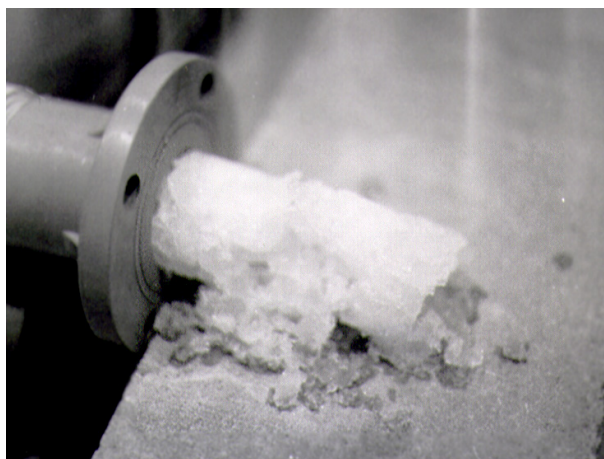
Figure 6. Snow noodle formed at porous wall in a water separator.
