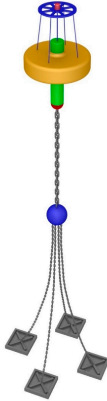
Figure 10. Graphic representation of a DEIM Point Absorber.
