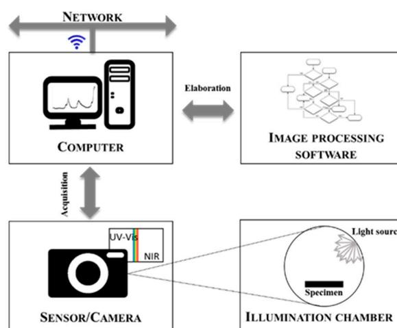
Figure 2. Elements of a computer vision (CV) system.
