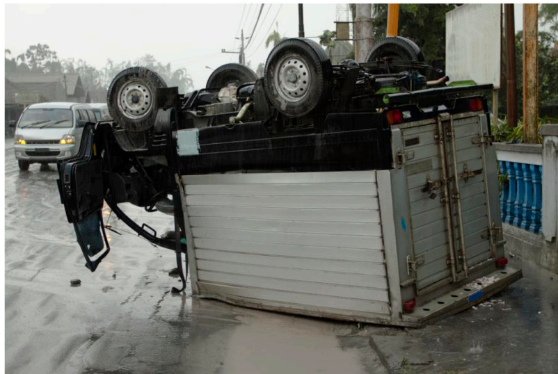
Figure 2. Vehicle accident attributed to reduced skid resistance after ashfall from Merapi volcano, Indonesia, 2010 [68].
