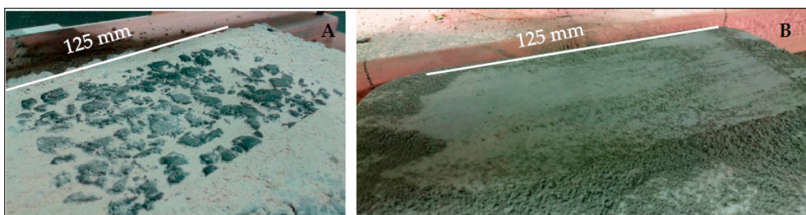
Figure 12. Dry ash displacement from the BPT slider-surface interface after 8 \times swings of the pendulum arm for (A) SMA and (B) airfield concrete. Dry ash was displaced from the surface more readily than wet ash. Note that white lines indicate length of slider contact path (i.e., 125 mm).
