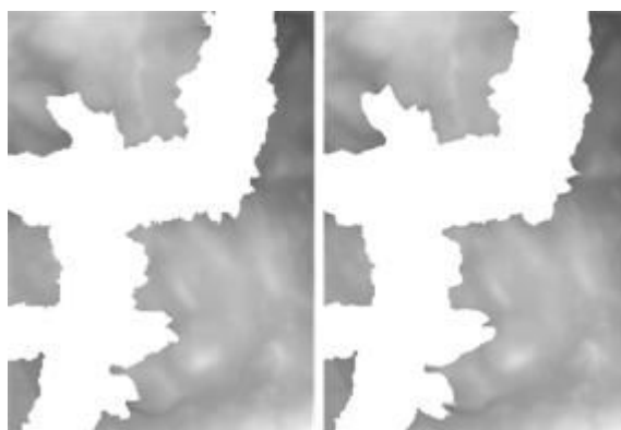
Figure 10. Results of canyon extractions performed on DTMs with the resolution of 8 (left) and 16 (right) meters.
