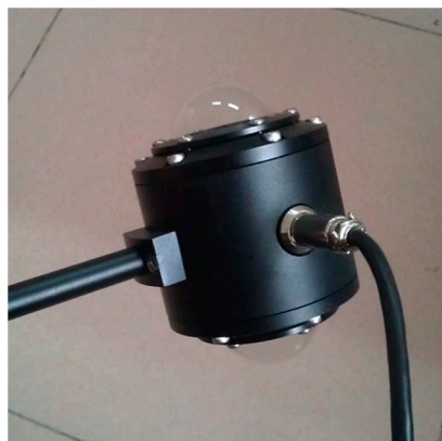
Figure 3. Developed spectral albedometer for one band.
