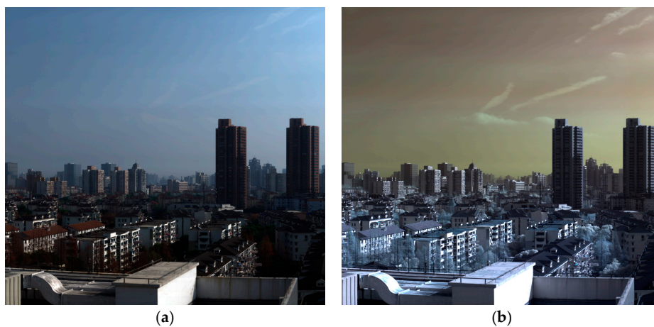
Figure 19. Correction results of the ground data using the proposed method. (a) RGB image in visible bands (R: 650 nm, G: 560 nm, B: 480 nm); (b) False-color RGB image in NIR bands (R: 800 nm, G: 890 nm, B: 960 nm).
