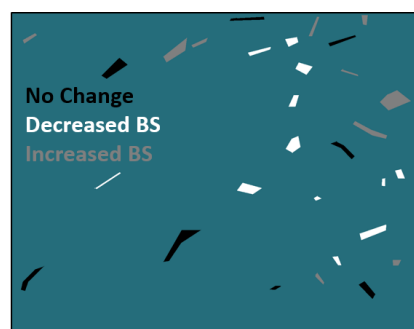
Figure 6. Test map used in the quantitative analysis of the performances. The black patches represent “no-change” areas, while grey and white patches represent “change” areas due to increased and decreased backscattering, respectively. The dark cyan background indicates the pixels that are not included in the test set.
