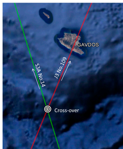
Figure 13. The cross-over location of Sentinel-3A Pass No.14 and Jason-3 Pass No.109 south of Gavdos Cal/Val site.
