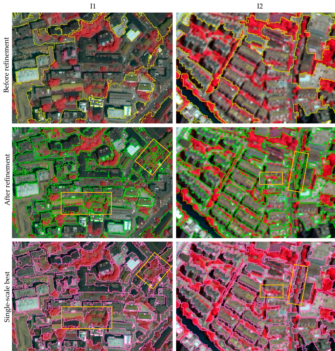
Figure 12. Comparison of sample segmentation results of test image I1 and I2 before refinement (the first row), after refinement (the second row), and the single-scale best segmentation result according to F -score (the third row), which are shown with yellow, green, and pink polygons, respectively. Four areas are highlighted for comparison using orange rectangles.
