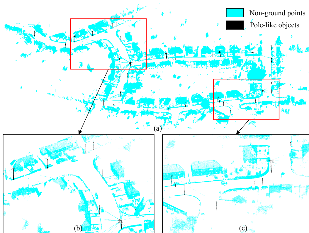
Figure 9. Results of PLOs extraction in Data I. (a) Non-ground points colored in cyan and PLOs colored in black; (b) view 1; (c) view 2.
