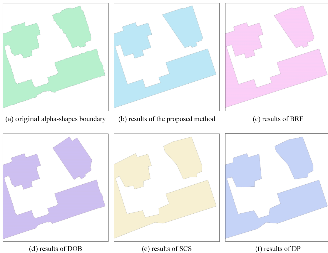
Figure 12. Zoom-in comparison of the regularization methods applied to ALS point clouds in the red box region of Figure 10. (a), original alpha-shapes boundary; (b–f), results of the proposed method, BRF [20], DOB [47], SCS [31], and DP [27] respectively.
