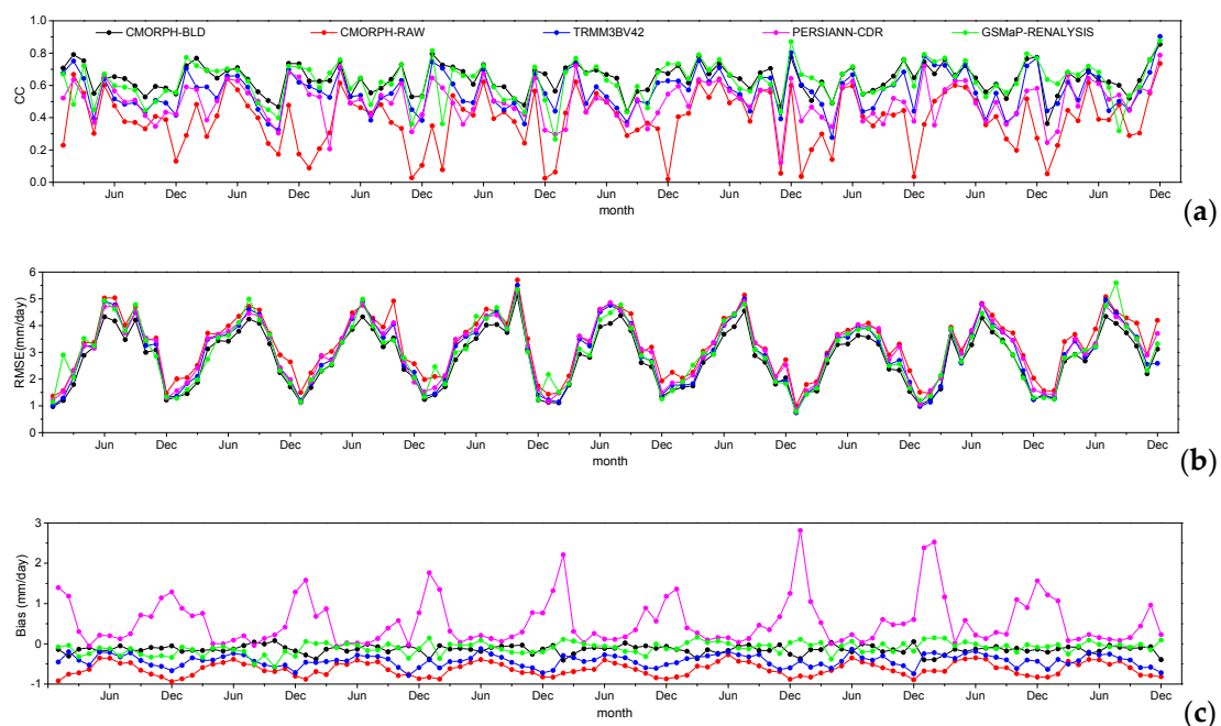
Figure 6. (a–c) denote the time series of the CC, RMSE and BIAS from a variety products spanning 2005 to 2013 over China, respectively.
