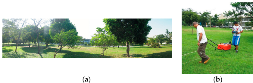
Figure 2. (a) Test site panoramic view; (b) Acquisition on the test site with 200 MHz antenna.
