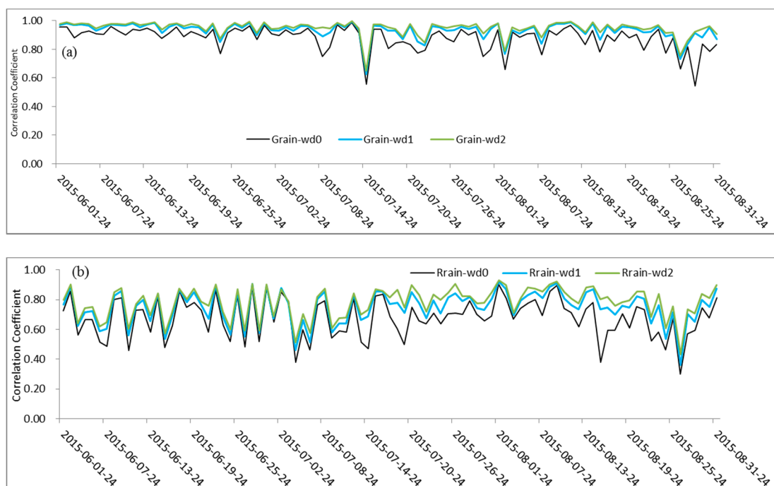
Figure 14. (a) Time series of correlation coefficients between the hydrological precipitation observations and gauge precipitation analysis (Grain); (b) time series of correlation coefficients between the hydrological precipitation observations and radar QPE (Rrain) and at the three sampling windows, wd0, wd1 and wd2, respectively, from June–August 2015.
