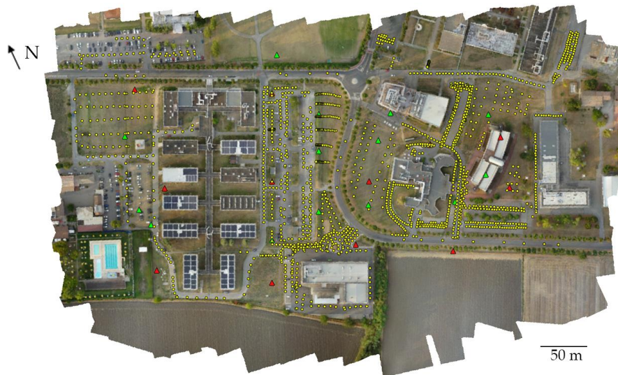
Figure 2. Location of the targets (ground control points (GCPs): red; checkpoints: green) and of the Digital Surface Model (DSM) checkpoints (yellow) on the orthophoto mosaic generated from one of the eight flights.
